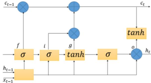
Figure 16. An LSTM cell with gates that helps data be processed sequentially
