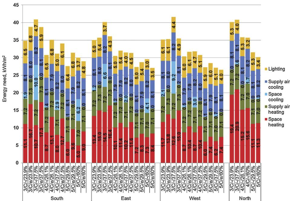
Fig. 13. Energy needs of final simulation cases for all zones. Insulation thicknesses determined in Section 3.4 are used.
