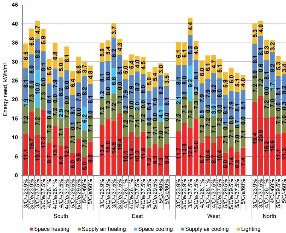
Figure 19 Energy needs of final simulation cases for all zones. Insulation thicknesses determined in Section 3.1.5 were used.
