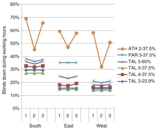
**Fig. 11** The effect of control principle, facade solution, orientation and climate on the time that blinds are down during working hours
