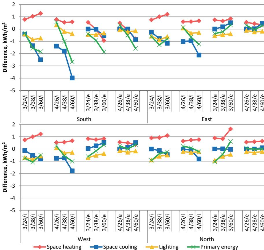
Figure 43 The difference of energy simulation results obtained with standard window models compared to simulations with detailed window models.
