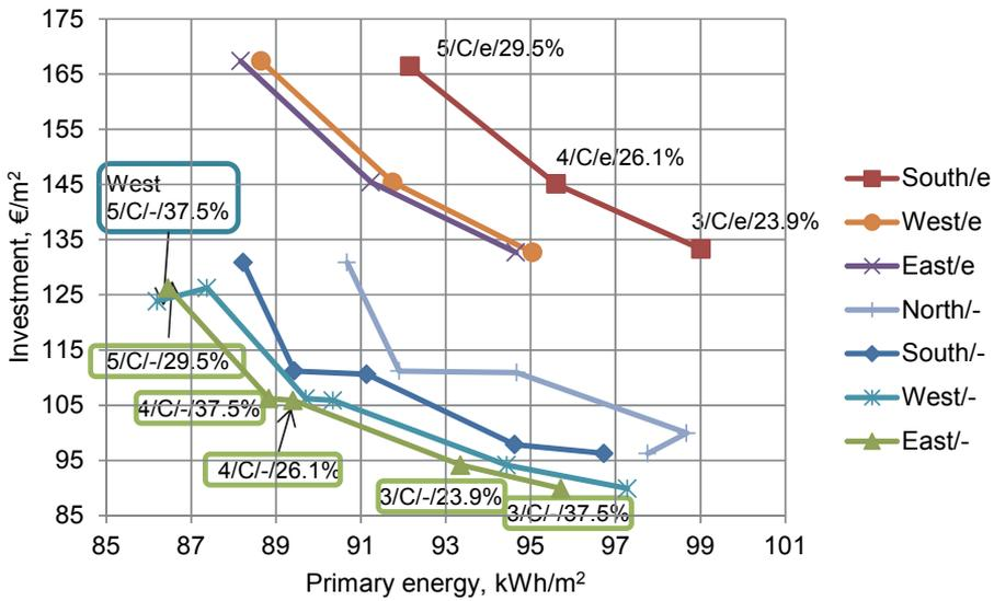
Figure 22 Investment and primary energy of final simulation cases. Three upper curves are with external shading (marked with e) and lower curves with internal blinds.
