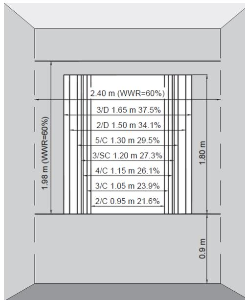
Figure 13 Window sizes of glazing variants (Variant codes correspond to Table 2, e.g. 2/C 0.95 m 21.6% means double, highly transparent window with width of 0.95 m and the window-to-wall ratio 21.6%). 2.4 m is the maximum width of the window providing WWR 60%.
