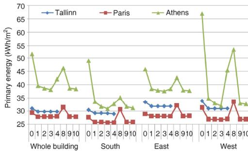
**Fig. 9** The primary energy use of control principles 1–4 and 8–10 in the climates of Tallinn, Paris and Athens. Control principles 8–10 were not simulated in the case of Tallinn
