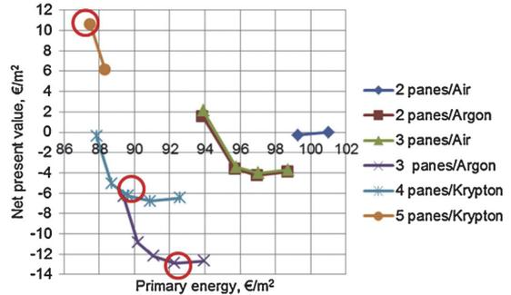
Fig. 12. Net present value and primary energy for the cases of Fig. 11. (For interpretation of the references to color in the text, the reader is referred to the web version of the article.)
