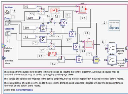
**Fig. 4** Macro for shading control in strategies 1–7 composed in IDA ICE. The description of elements is shown in Table 5. The components used for control strategies 1–7 are shown in the figure, whereas none of the strategies contain all elements
