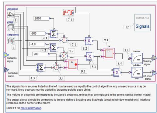
**Fig. 5** Macro for shading control in strategies 8–10 composed in IDA ICE. The description of elements is shown in Table 5. The components necessary to describe control strategies 8–10 are shown in the figure. Some of the macro components are also shown in Fig. 4 and their labels are the same
