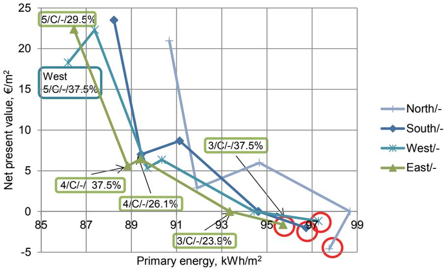
Figure 23 Net present value and primary energy of final simulation cases without external shading.
