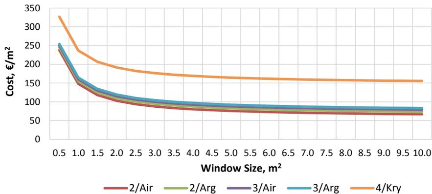
Figure 14 Specific window cost as a function of window size.
