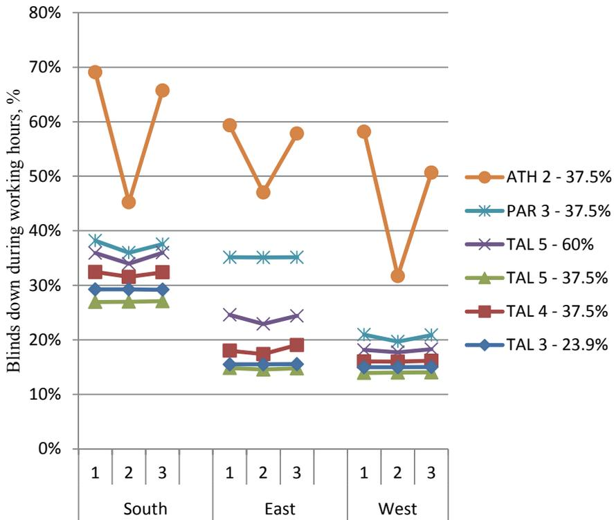
Figure 32 The effect of control principle, facade solution, orientation and climate on the time that blind are down during working hours.
