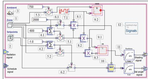
**Fig. 12** The macro of optimal control principle in Athens (control principle no. 3 in Table 4 and Table 5)
