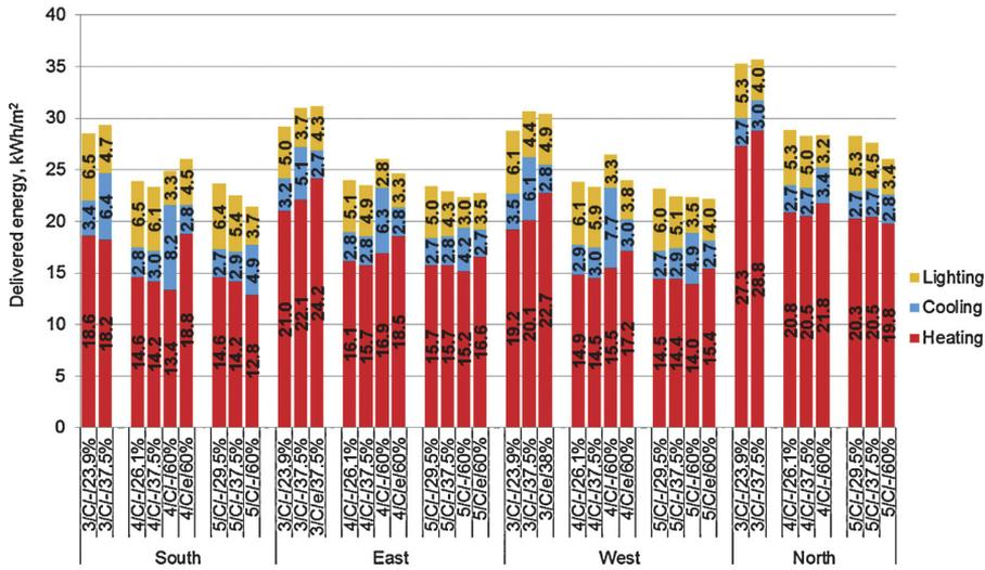
Fig. 9. Delivered energy results of the cases used to determine optimal WWR with initial fixed insulation thickness (200 and 300 mm for 3 and 4 pane respectively). Delivered energy is given in each zone as a function of window type, external shading, orientation and window size. Case codes are described in Table 2, e.g. 3/Ci-/23.9% means 3-pane, clear solar protection glass, no external shading and WWR = 23.9%.
