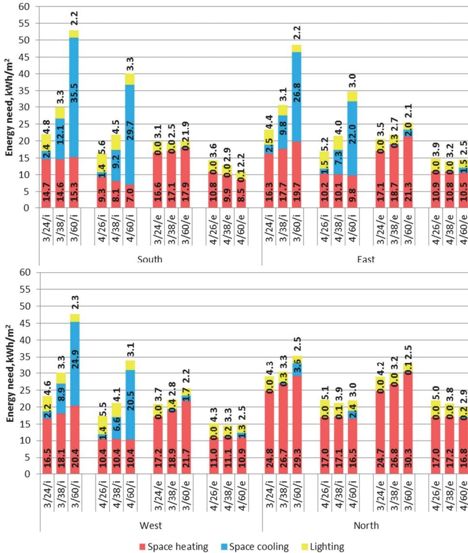
Figure 6 Energy needs of all studied cases. External wall insulation thicknesses 150 and 200 mm were used with triple and quadruple windows respectively. The results are given as a function of window type, WWR and type of shading e.g. 3/24/i means a case with triple windows, WWR 24% and internal shading. „e“ means external shading.
