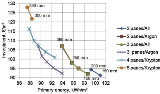
Fig. 11. Investment cost and primary energy of different glazing (all without external shading) and external wall insulation cases. Insulation thicknesses from left to right 150, 200, 250, 300 and 390 mm if not otherwise specified.
