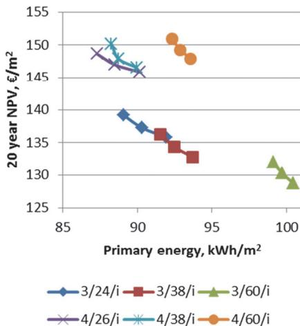
Figure 5 The 20 year NPV and primary energy depending on the external wall mineral wool thickness. The points of each facade represent 150, 200 and 250 mm from right to left respectively. The case codes illustrate window type, WWR and type of shading e.g. 3/24/i means a case with triple windows, WWR 24% and internal shading.
