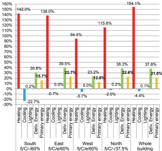
Figure 25 Energy use fluctuation of the most energy-efficient cases
