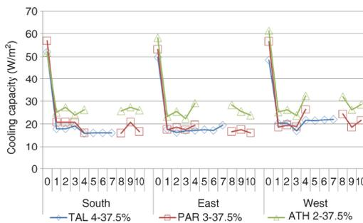
**Fig. 14** The cooling capacities of different control principles in different climates
