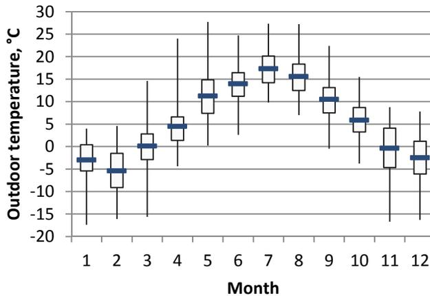
Figure 5 The minimum, maximum and average temperatures of each month of Estonian test reference year. The average values are indicated with dark markers and the 25th and 75th percentiles are also presented.
