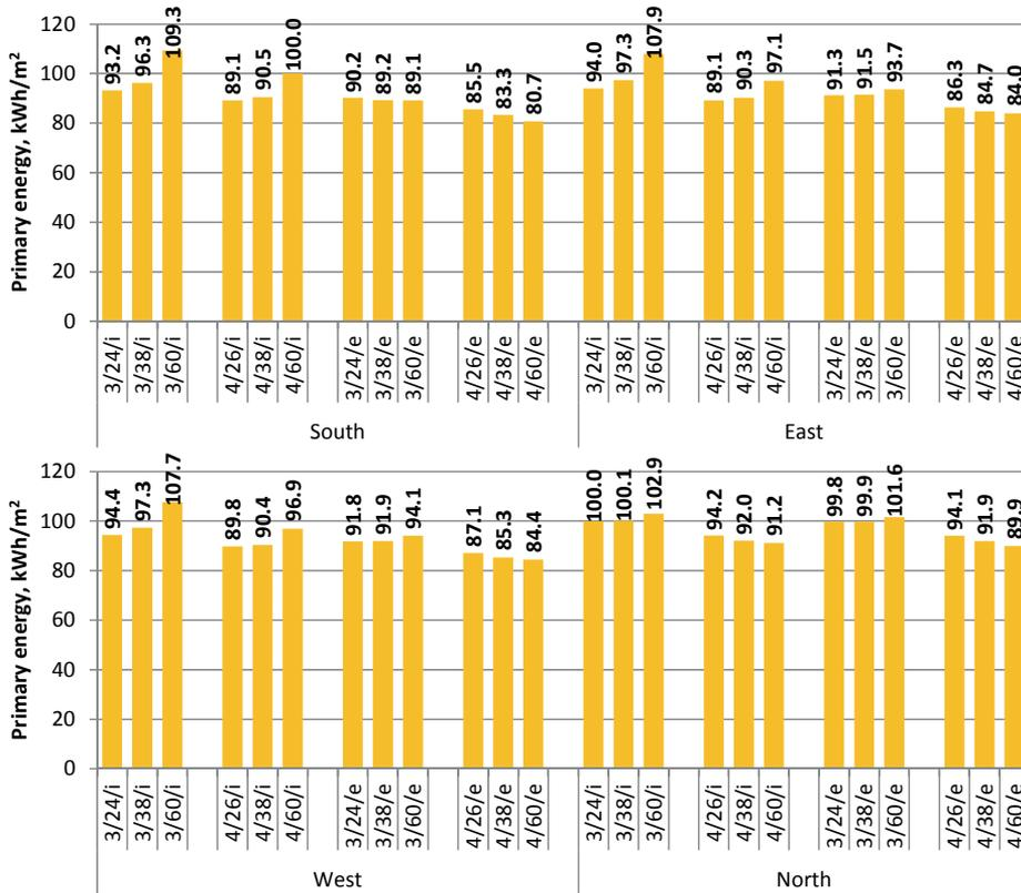
Figure 41 Primary of all studied cases. The results are given as a function of window type, WWR and type of shading e.g. 3/24/i means a case with triple windows, WWR 24% and internal shading. „e“ means external shading.
