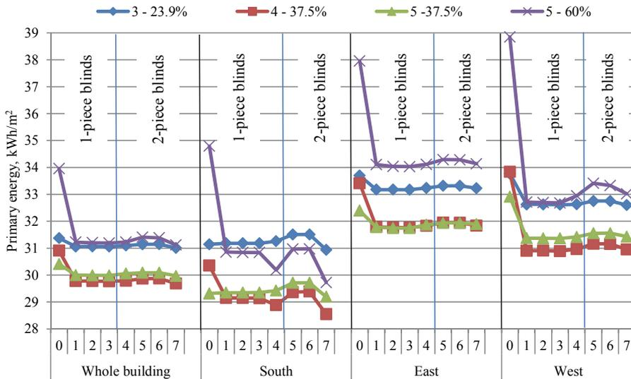
Figure 27 The primary energy use of control principles 1-7 in the climate of Tallinn. Case 0 stands for internal venetian blinds. Only the energy for space heating and cooling, supply air heating and cooling and electric lighting are included.
