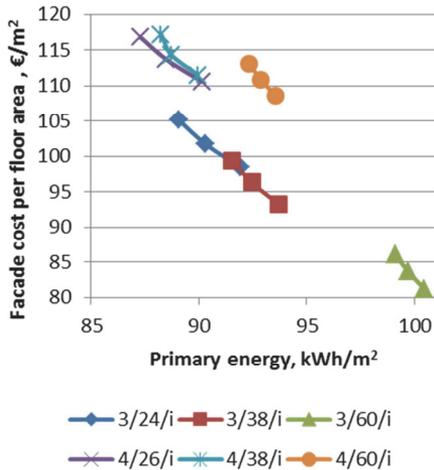
Figure 4 The facade cost and primary energy depending on the external wall mineral wool thickness. The points of each facade represent 150, 200 and 250 mm from right to left respectively. The case codes illustrate window type, WWR and type of shading e.g. 3/24/i means a case with triple windows, WWR 24% and internal shading.
