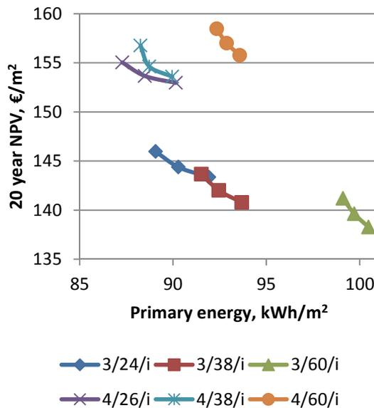
Figure 39 The 20 year NPV and primary energy depending on the external wall mineral wool thickness. The points of each facade represent 150, 200 and 250 mm from left to right respectively. The case codes illustrate window type, WWR and type of shading e.g. 3/24/i means a case with triple windows, WWR 24% and internal shading.
