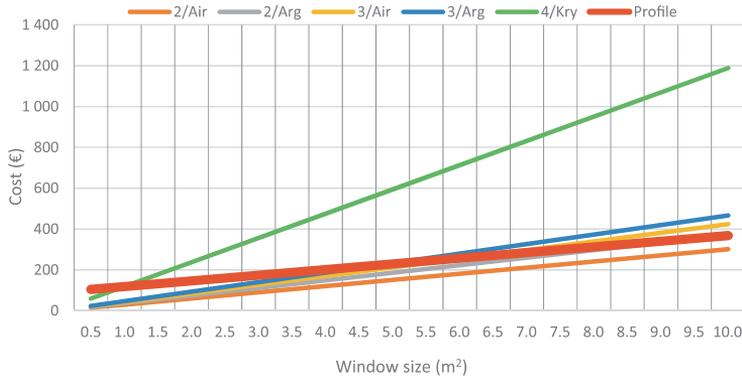
Fig. 5. The cost of window components (profile and glazing) per window size.
