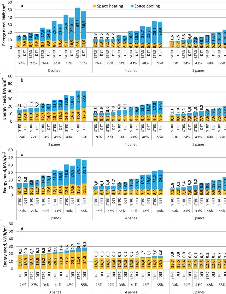
Figure 37 Space heating and cooling needs in the (a) South, (b) East, (c) West and (d) North oriented zones in case of standard and detailed window models. Code: STRD – standard window model, DET – detailed window model; 24% means window-to-wall ratio 24%.
