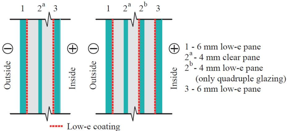
Figure 8 The construction of triple and quadruple glazing and positioning of low-emissivity layers. The same glazing types were also studied in [70].
