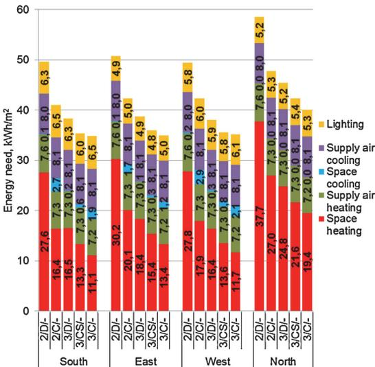
Fig. 6. Energy need in zones with highly transparent and solar protection windows with minimum size according to the daylight criterion of 2%.
