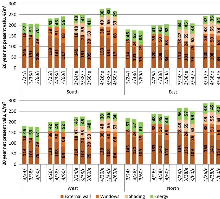
Figure 42 Net present value of all studied cases per floor area of respective zones. The results are given as a function of window type, WWR and type of shading e.g. 3/24/i means a case with triple windows, WWR 24% and internal shading. „e“ means external shading.
