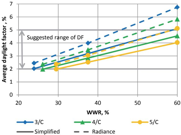
Figure 12 The average daylight factors calculated with the simplified formula and with IDA-ICE coupled with Radiance. Code: 3/C – triple highly transparent window; 4/C – quadruple highly transparent window; 5/C – quintuple highly transparent window.
