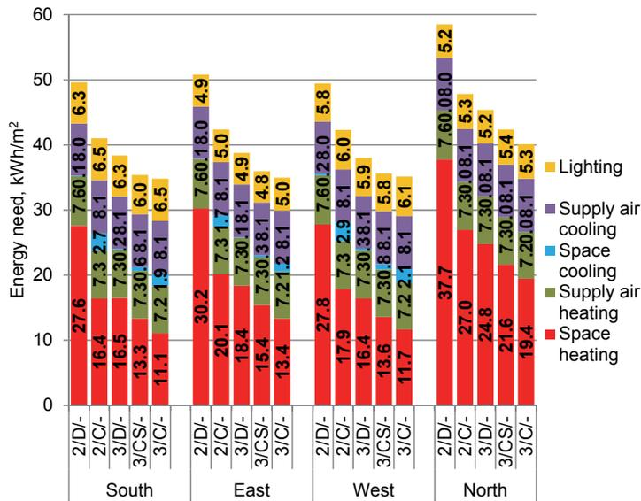
Figure 15 Energy need in zones with highly transparent and solar protection windows with minimum size according to the daylight criterion of 2%. Case codes: number 2 or 3 means double or triple panes, D, C and SC mean tinted solar protection, clear highly transparent and clear solar protection glazing respectively and “-“ represent internal shading.
