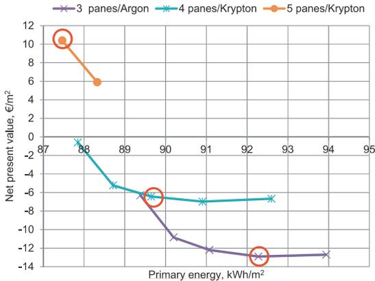
Fig. 8. NPV and Primary Energy performance for selected combinations. Insulation thicknesses from right to left are per sequential points are 150, 200, 250, 300 and 390 for triple and quadruple glazing. Insulation thicknesses from right to left for quintuple glazing are 300 and 390.
