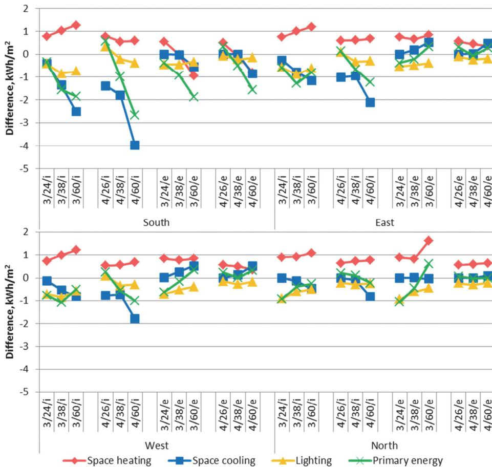
**Figure 9** The difference of energy simulation results obtained with standard window models compared to simulations with detailed window models. The results are given as a function of window type, WWR and type of shading e.g. 3/24/i means a case with triple windows, WWR 24% and internal shading. „e“ means external shading.
