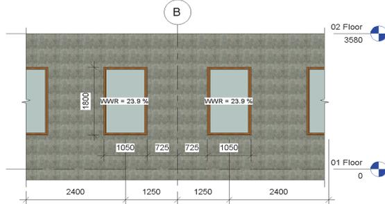
B1. Cost-effective solution with higher cooling load than recommended solution: triple glazing ( $U_{gl}=0.57 \text{ W}/(\text{m}^2\cdot\text{K})$ ,  $\text{SHGC}=0.49$ ,  $\tau_{vis}=0.70$ ), WWR 37.5% (60% in North façade) and 150 mm thick insulation ( $U=0.20 \text{ W}/(\text{m}^2\cdot\text{K})$ ). Heating capacity 14-16  $\text{W}/\text{m}^2$ , 19  $\text{W}/\text{m}^2$  in the North façade; sensible cooling capacity 53-62  $\text{W}/\text{m}^2$  (except North façade).
