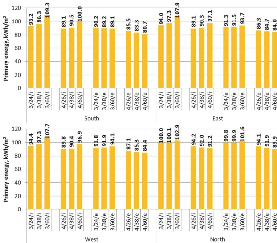
Figure 7 Primary of all studied cases. The results are given as a function of window type, WWR and type of shading e.g. 3/24/i means a case with triple windows, WWR 24% and internal shading. „e“ means external shading.
