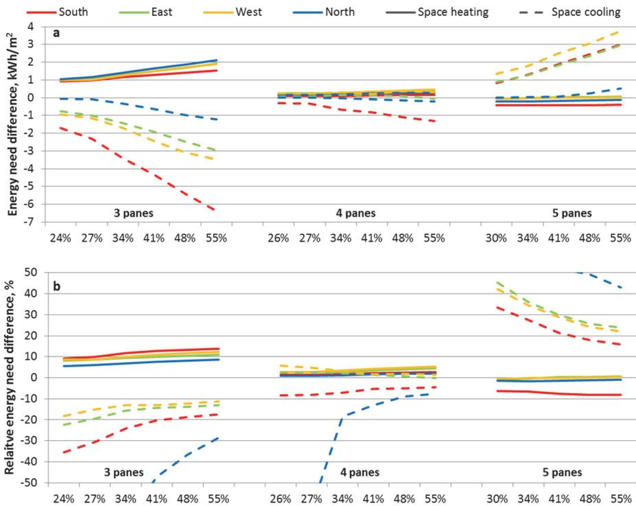
Figure 38 Detailed window models space heating and cooling need difference from standard window models in zones with different orientations and window types. (a) energy need of detailed window models has been deducted from standard window models respective value; (b) value shows how much the energy need with detailed glazing differs from standard glazing. Code: 24% means window-to-wall ratio 24%.
