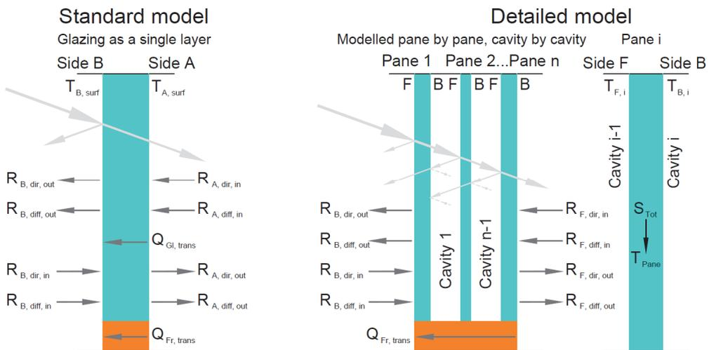
**Figure 2** The calculated variables of standard and detailed glazing models in IDA-ICE. Code: T – temperature of a surface or pane; R – diffuse/direct radiation in/out of a pane/glazing; Q – heat transmission of glazing/frame from surface to surface; S – total absorption heat flux.
