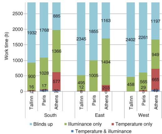
**Fig. 10** The illustration of shading need on different facades in all climates in the case of control principle no. 1
