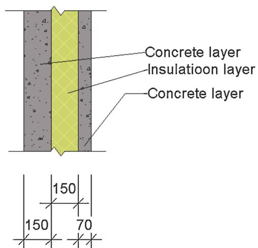
**Fig. 3.** Section of external wall, the thickness on insulation varies by cases.
