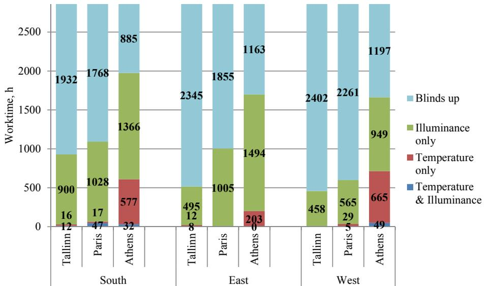
Figure 31 The illustration of shading need on different facades in all climates in case of control principle no 1.
