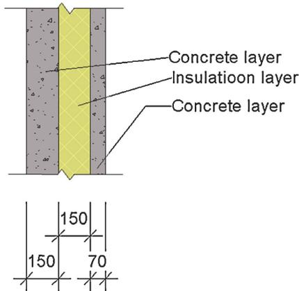
Fig. 3. Gross section of the typical exterior wall.
