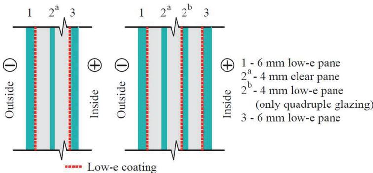
**Figure 3** The construction of triple and quadruple glazing and positioning of low-emissivity layers. The same glazing types were also studied in (Thalfeldt, Kurnitski, and Voll [submitted]).
