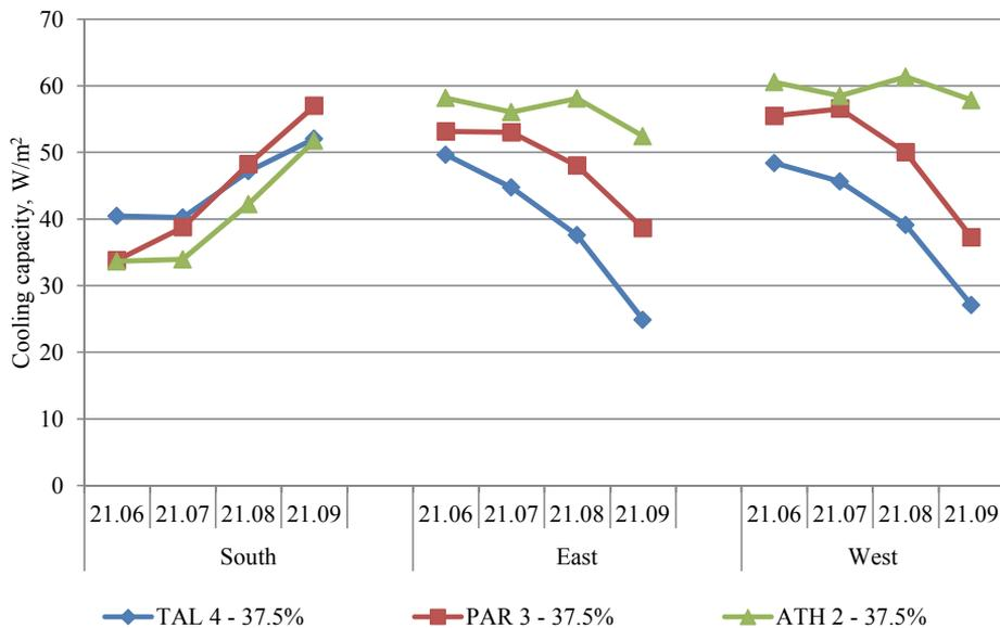
Figure 36 The cooling capacities in different climates depending on the design day.
