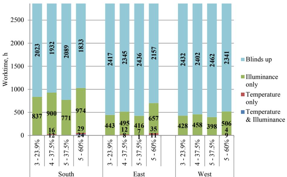
Figure 28 The illustration of shading need on different facades in the climate of Tallinn in case of control principle no 1.
