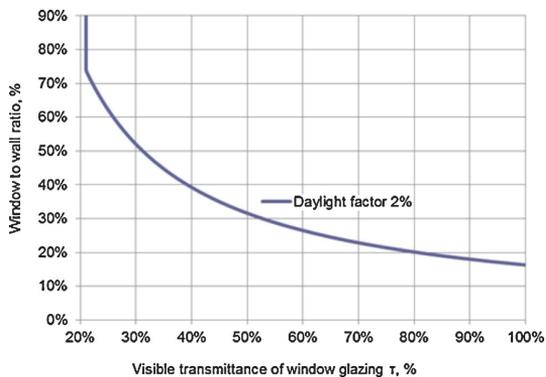
**Fig. 4.** Minimum window to wall ratio depending on visible transmittance of window glazing.
