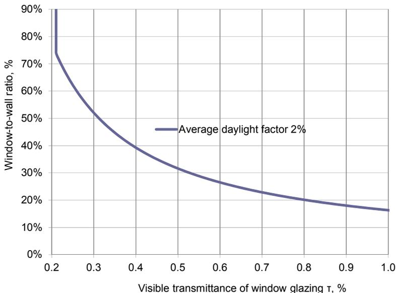
Figure 11 Minimum window-to-wall ratio depending on visible transmittance of glazing in case of an office room consisting of two 2.4 meters wide modules.
