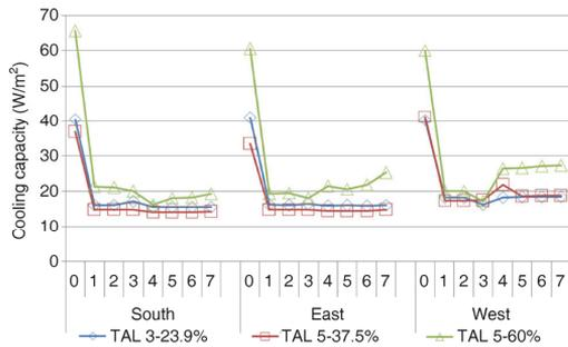
**Fig. 13** The cooling capacities of different control principles in Tallinn cases with triple and quintuple windows. The case quadruple glazing is shown in Fig. 14
