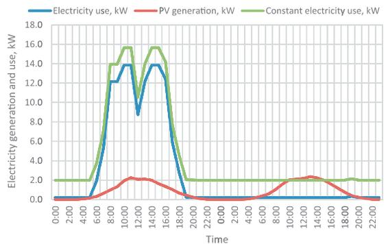
**Fig. 11.** An example of load matching for a working day, 29 June 2012, and non-working day, 30 June 2012.
