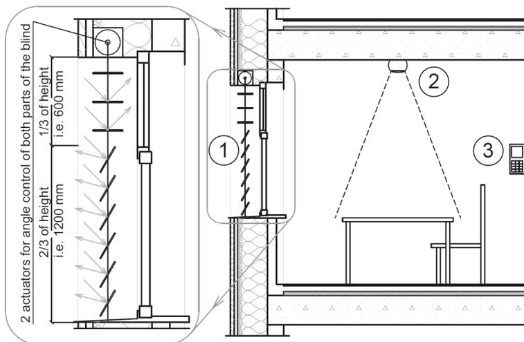
Figure 10 Cross-section of an office room. 1 – Motorized external venetian blind with two actuators for changing position and slat angle, 2- multisensor for detecting occupancy and measuring illuminance at desktop, 3 – control panel with built in temperature sensor
