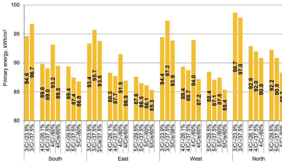
Figure 16 Primary energy results of the cases used to determine optimal WWR with initial fixed insulation thickness (200 and 300 mm for 3 and 4 pane respectively). Primary energy is given in each zone as a function of window type, external shading, orientation and window size. Case codes are described in Table 2, e.g. 3/C/-/23.9% means 3-pane, clear solar protection glass, no external shading and WWR=23.9%.
