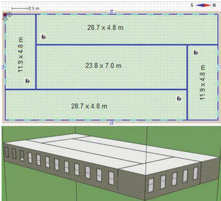
**Figure 1** The generic model of single floor of an office building constructed with 2.4 m room module – plan and 3D view. The same floor plan was used in (Thalfeldt et al. 2013).
