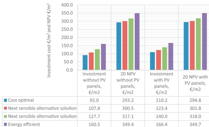
**Fig. 12.** Comparison of selected cases with and without PV panels.
