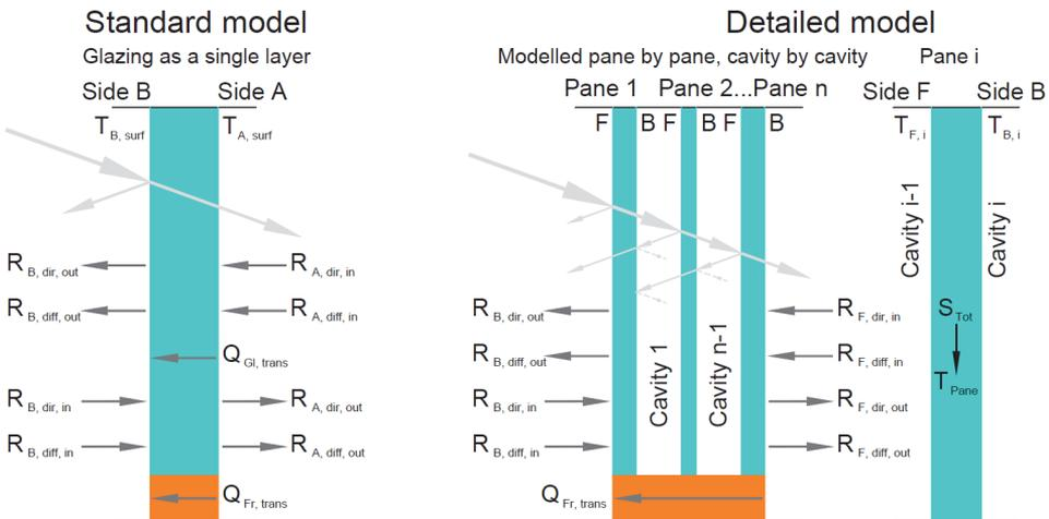
Figure 6 The calculated variables of standard and detailed glazing models in IDA-ICE. Code: T – temperature of a surface or pane; R – diffuse/direct radiation in/out of a pane/glazing; Q – heat transmission of glazing/frame from surface to surface; S – total absorption heat flux.
