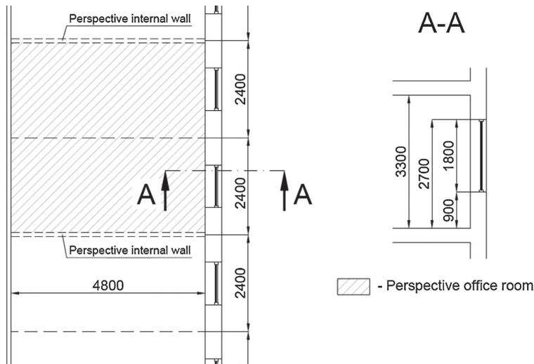
**Fig. 2.** Floor plan of the open plan office module (2.4 m) and the section showing window and room height.
