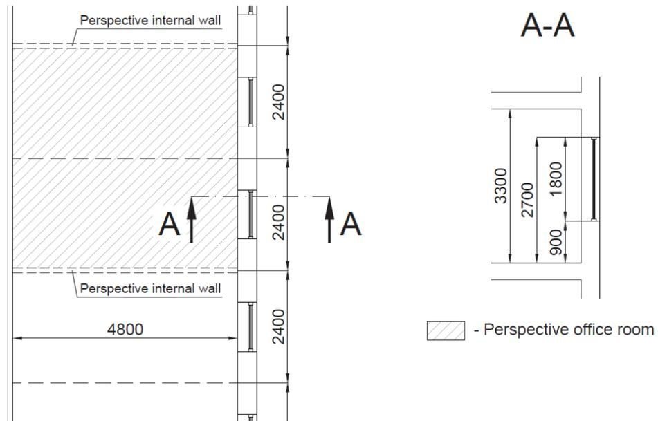
Figure 3 Floor plan of the open plan office module (2.4 m) and the section showing window and room height.
