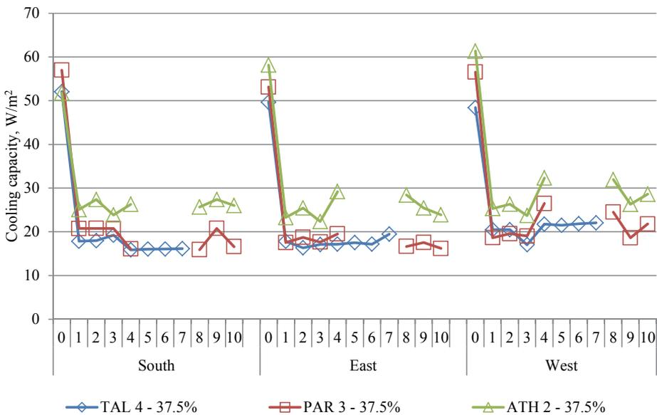
Figure 35 The cooling capacities of different control principles in different climates.
