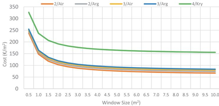
Fig. 6. Specific window cost as a function of window size.
