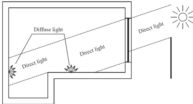
Figure 4 Daylight calculation principles of IDA-ICE.
