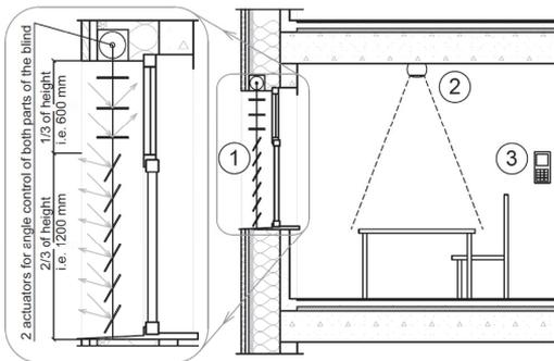
**Fig. 3** Cross-section of an office room. 1: motorized external venetian blind with two actuators for changing position and slat angle, 2: multisensor for detecting occupancy and measuring illuminance at desktop, 3: control panel with built in temperature sensor
