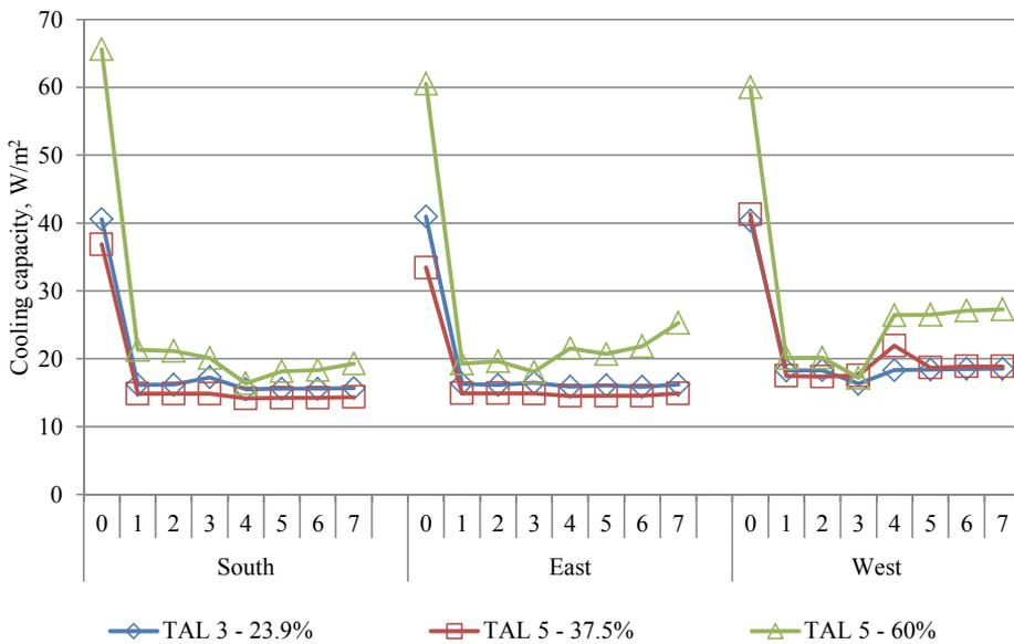
Figure 34 The cooling capacities of different control principles in Tallinn cases with triple and quintuple windows. The case with quadruple glazing is shown in Figure 35.
