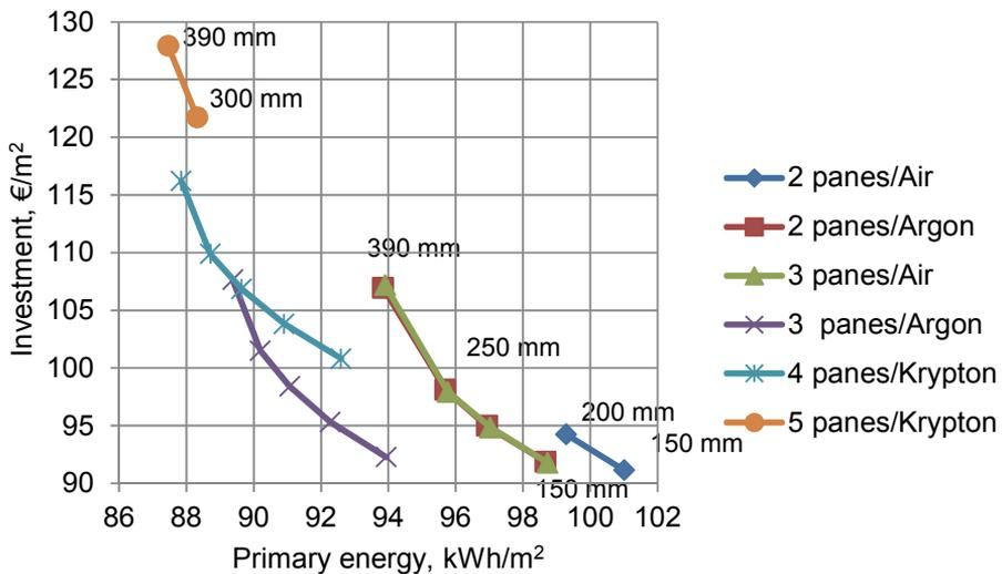
Figure 17 Investment cost and primary energy of different glazing (all without external shading) and external wall insulation cases. Insulation thicknesses from left to right 150, 200, 250, 300 and 390 mm if not otherwise specified.
