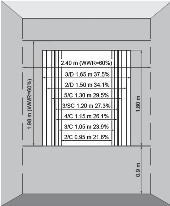
Fig. 5. Window sizes of glazing variants (variant codes correspond to Table 2, e.g. 2/C 0.95 m 21.6% means double, highly transparent window with width of 0.95 m and the window-to-wall ratio 21.6%). 2.4 m is the maximum width of the window providing WWR 60%.
