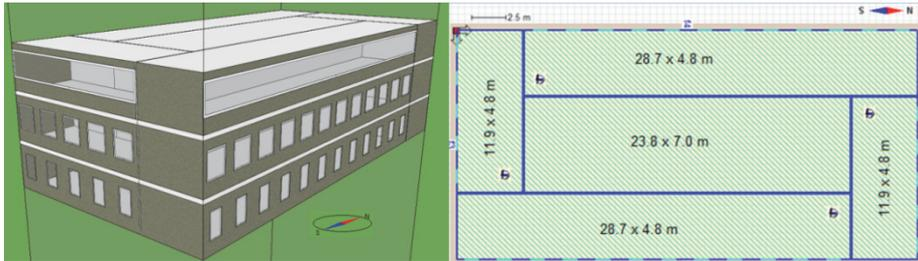
Figure 1 The generic model of single floor of an office building constructed with 2.4 m room module – plan and 3D view. The locations of workplaces used for control of lighting are marked in the plan.
