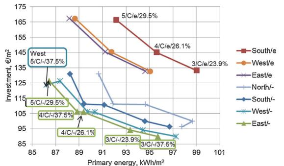
Fig. 16. Investment and primary energy of final simulation cases. Three upper curves are with external shading (marked with e) and lower curves with more cases without.
