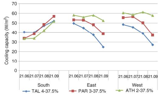
**Fig. 15** The cooling capacities in different climates depending on the design day
