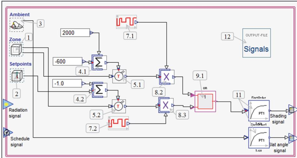
Figure 29 The macro of optimal control principle in Tallinn and Paris (control principle no 4 in Table 11).
