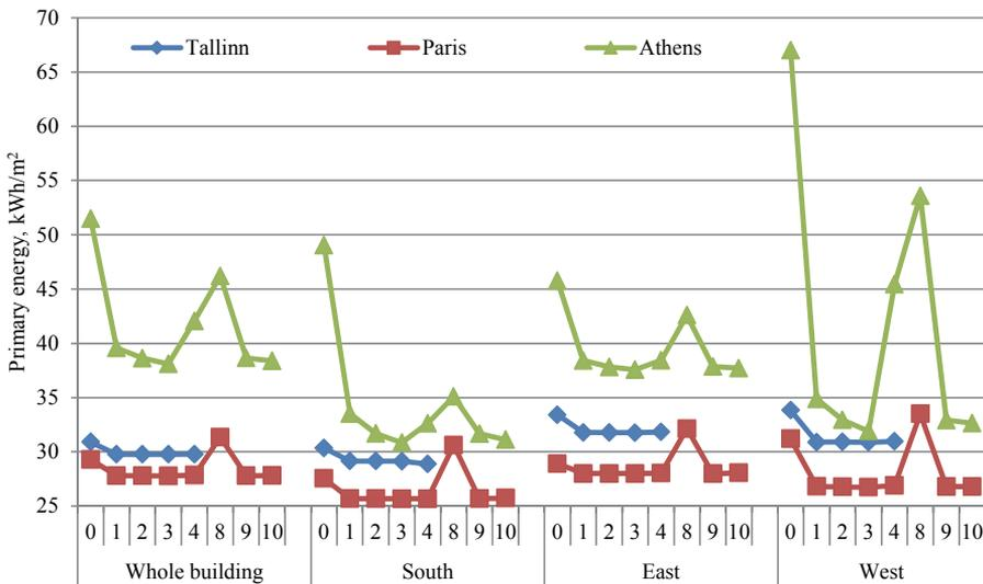
Figure 30 The primary energy use of control principles 1-4 and 8-10 in the climates of Tallinn, Paris and Athens. Control principles 8-10 were not simulated in case of Tallinn. Only the energy for space heating and cooling, supply air heating and cooling and electric lighting are included in the graph.
