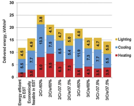
Fig. 21. Delivered energy in Paris. In two first cases the cost effective and most energy efficient façade solutions in Estonian climate are used. In other cases U-values were 1.1 for double glazing, 0.6 for triple glazing and 0.2 for external walls.
