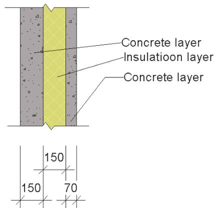
Figure 7 Gross section of the typical exterior wall.
