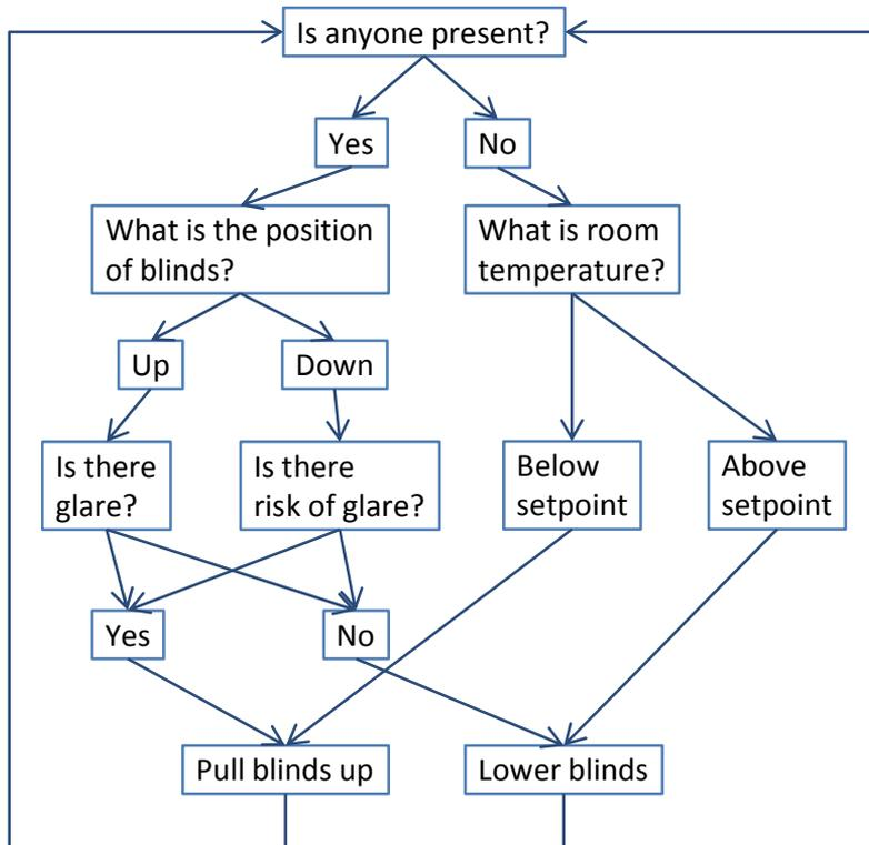
Figure 44 Description of control algorithm suitable for dynamic external blinds in an office building located in a cold climate.
