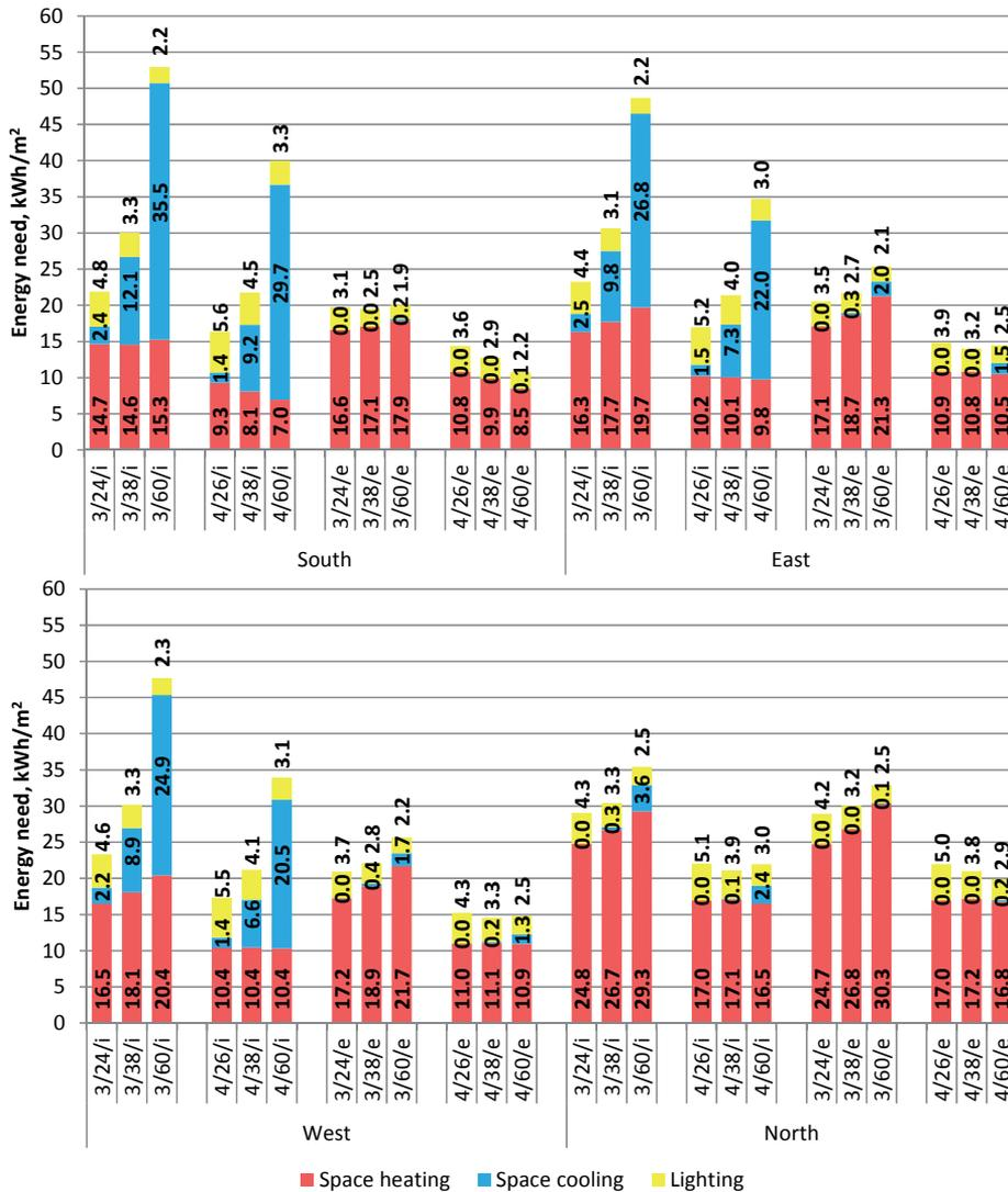
Figure 40 Energy needs of all studied cases. The results are given as a function of window type, WWR and type of shading e.g. 3/24/i means a case with triple windows, WWR 24% and internal shading. „e“ means external shading.
