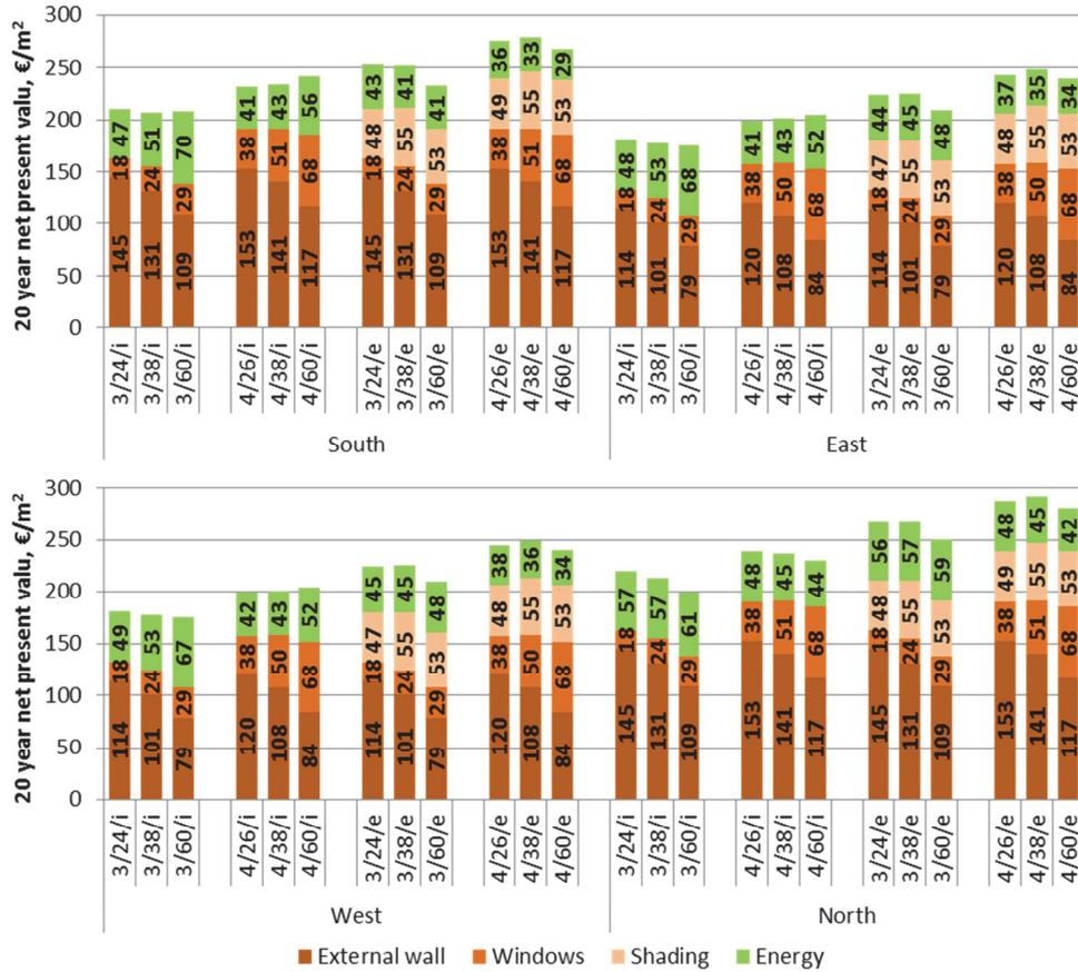
Figure 8 Net present value of all studied cases per floor area of respective zones. The results are given as a function of window type, WWR and type of shading e.g. 3/24/i means a case with triple windows, WWR 24% and internal shading. „e“ means external shading.
