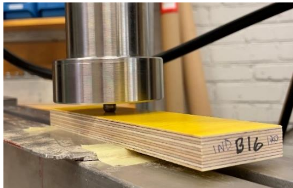
Figure 3.21. EN 1534 Brinell test procedure
