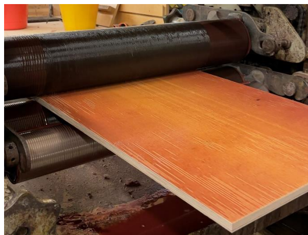
Figure 3.4. Gluing using roller- coater Black Bros 22-D
