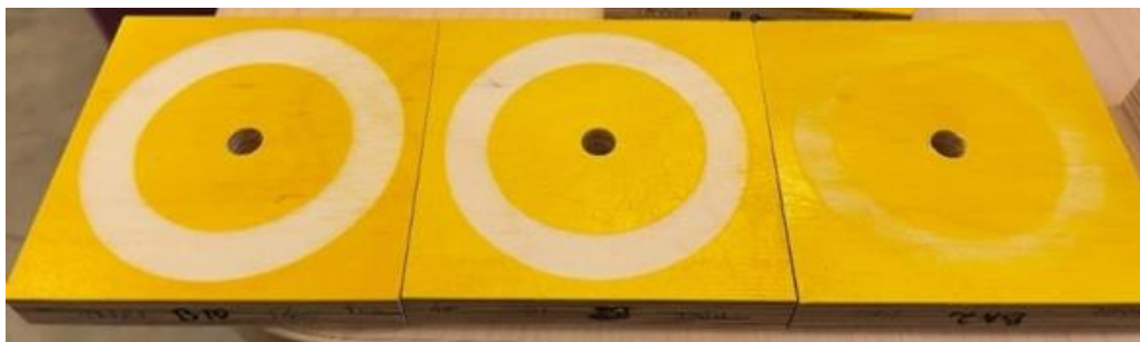
Figure 4.9. Taber abrasion test example 800, 400, 100 revolutions respectively
