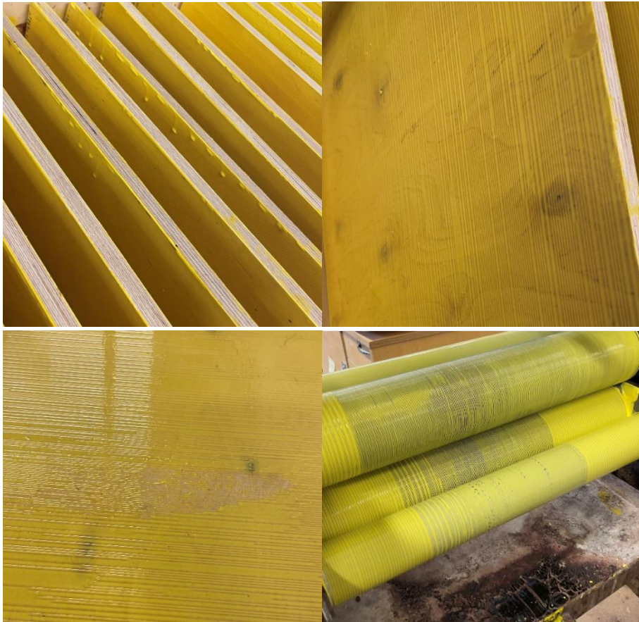
Figure 3.14. S2 120 spread rate, set to dry before press, bad spread issues
