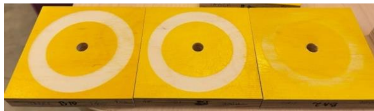
Figure 4.8. Unveneered scratch test average coefficient of friction (COF)
