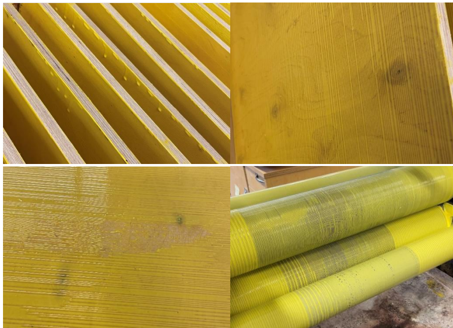
Figure 3.14. S2 120 spread rate, set to dry before press, bad spread issues
