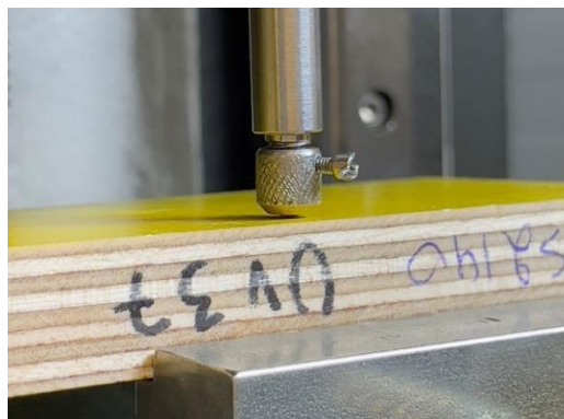
Figure 3.22. First attempt using a steel ball instead of cone
