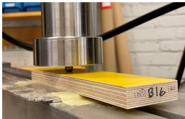
Figure 3.21. EN 1534 Brinell test procedure
