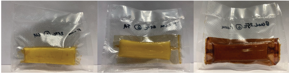
Figure S4. Gouda cheese packed in CH, TA:CH and CE:CH biofilms (from left to right).
