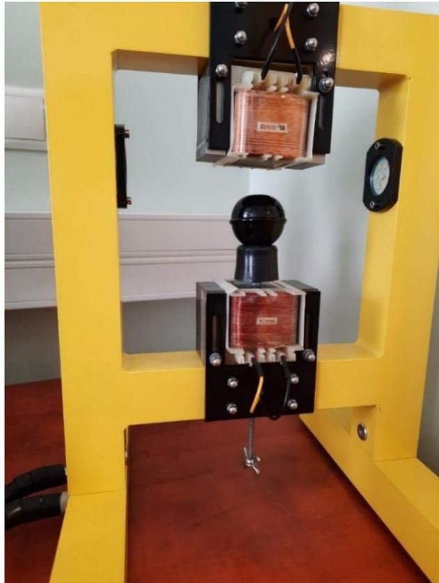
Figure 1. Experimental setup with the metallic sphere on the resting platform
