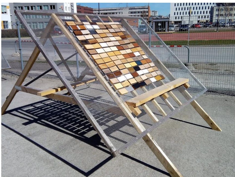
Figure 3.3. The stand of specimens in TalTech (Southern exposure, 59°23'50.6"N 24°39'24.0"E)
