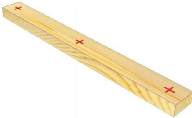
Figure 3.5. Marking of the colour measuring spots (Brischke et al , 2014)
