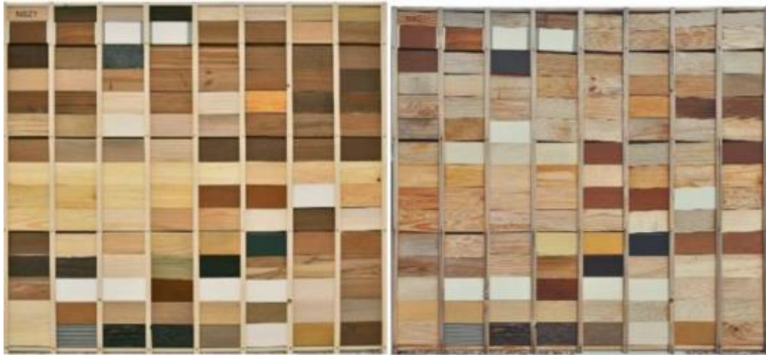
Figure 4.2 Experimental samples during natural weathering in San Michele, Italy (southern exposure, vertical stand) (Sandak et al , 2018c)
