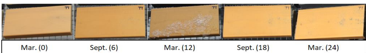
Figure 4.21. Visual colour change of Accoya (matt) (Legend: Calendar Month (Time of Exposure in Months))
