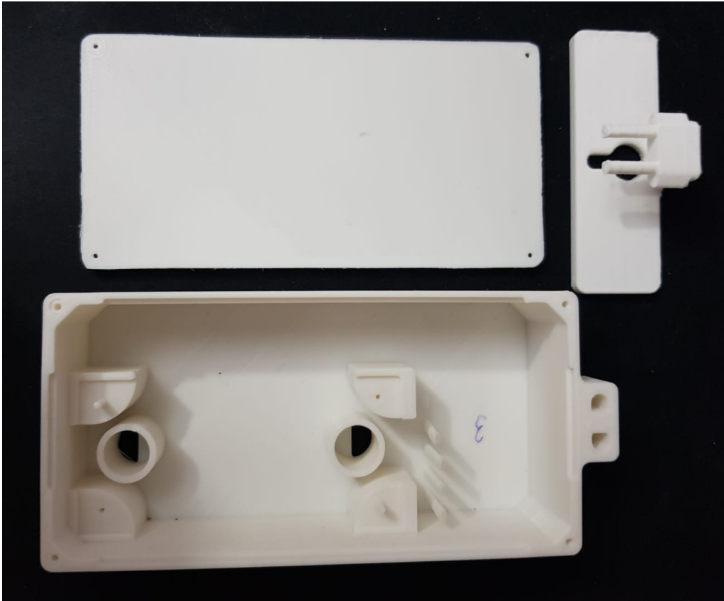
Figure 18 3D printed electronic enclosure design-1
