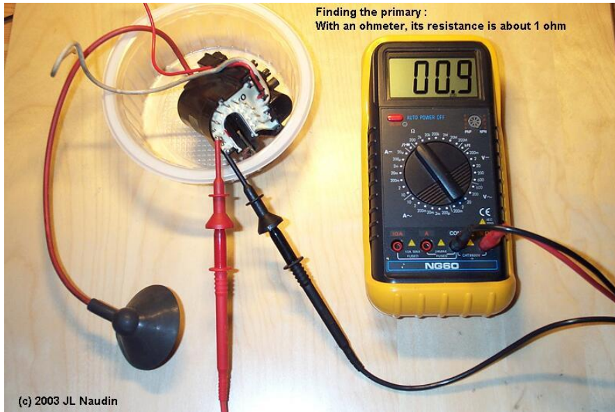
Figure 13 Setup to find the Primary pins in FBT.
