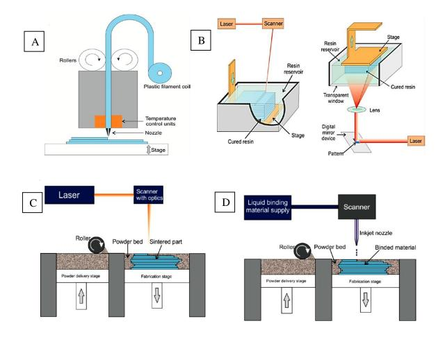
Figure 2. A – Schematic of an FDM 3D printer, B – Schematic of an SLA 3D printer (left – direct writing, right – mask-based writing), C – Schematic of an SLS 3D printer, D – Schematic of an inkjet printing apparatus [25].
