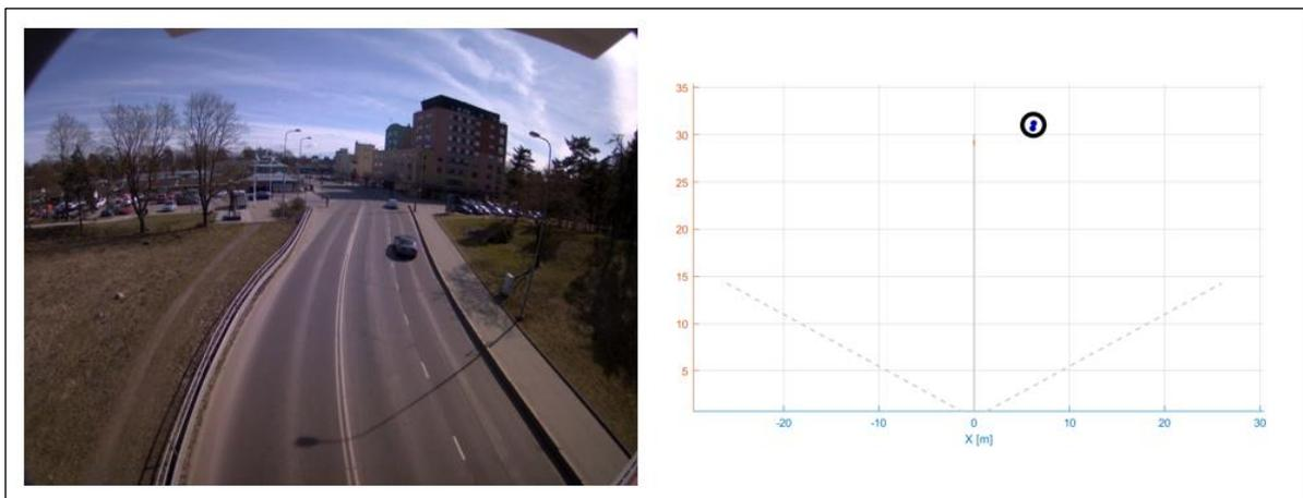
Figure 38. Visual data and corresponding radar output
