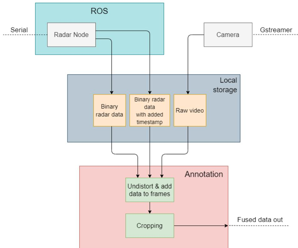
Figure 15. Block diagram of ROS flow
