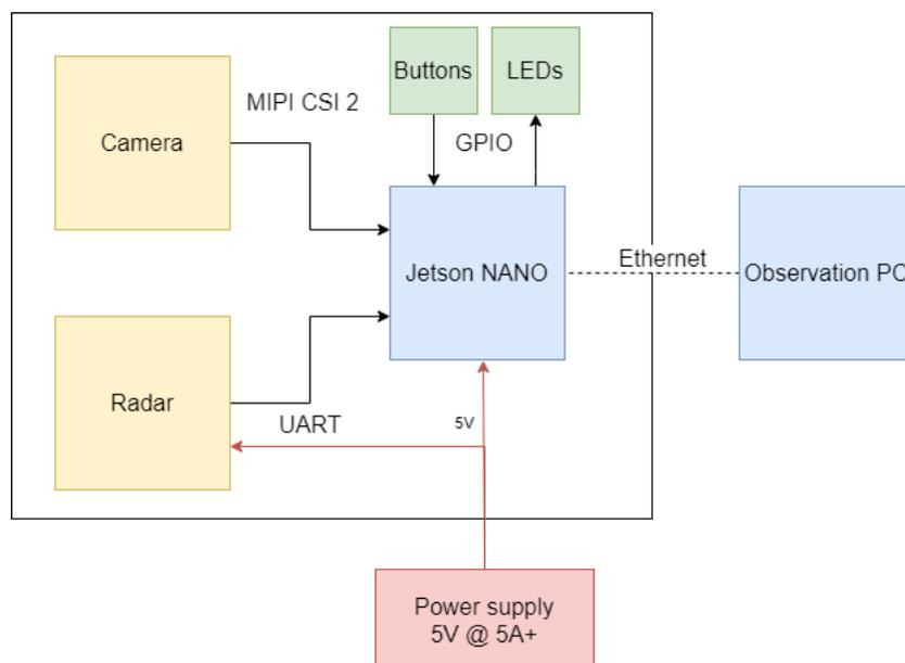
Figure 13. Hardware connectivity diagram
