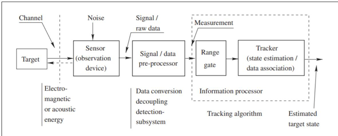
Figure 5. Object tracking system block diagram [25]
