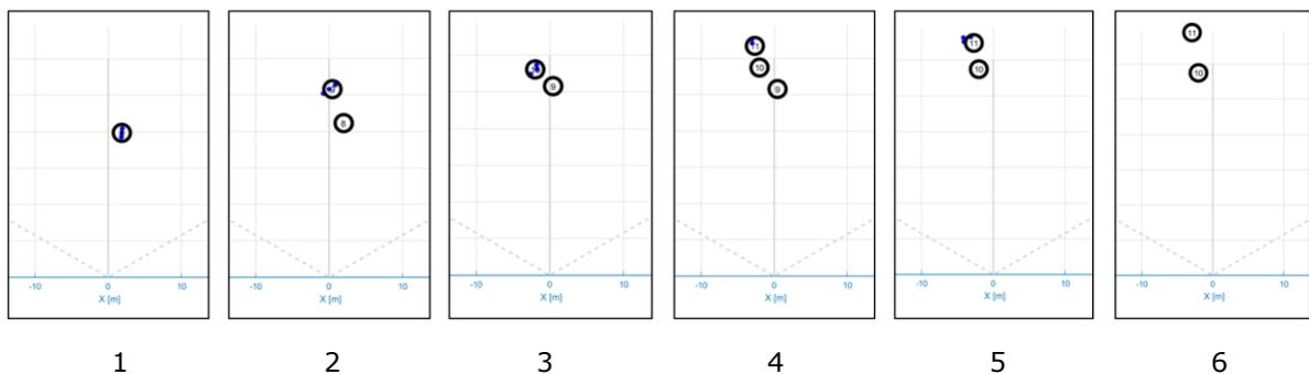
Figure 34. Fragmentation issue due to low acceleration limits
