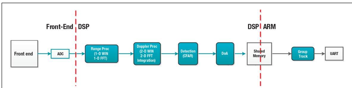
Figure 19. Detection, tracking and visualization signal-processing chain [5]
