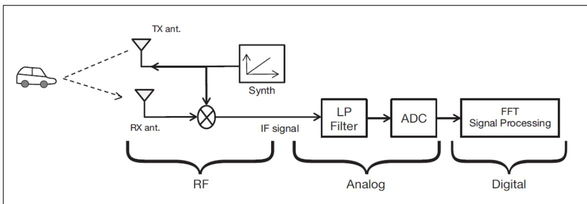
Figure 8. Block diagram of radar components [31]
