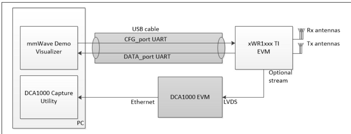
Figure 16. Connectivity between mmWave Demo Visualizer and EVM [48]
