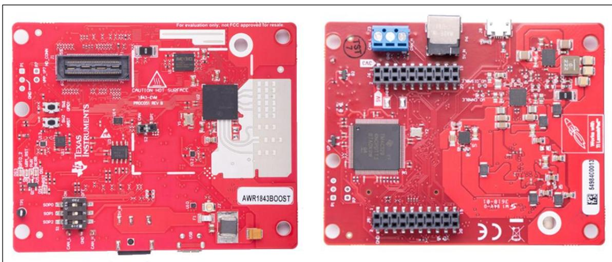
Figure 10. Front and rear sides of the EVM
