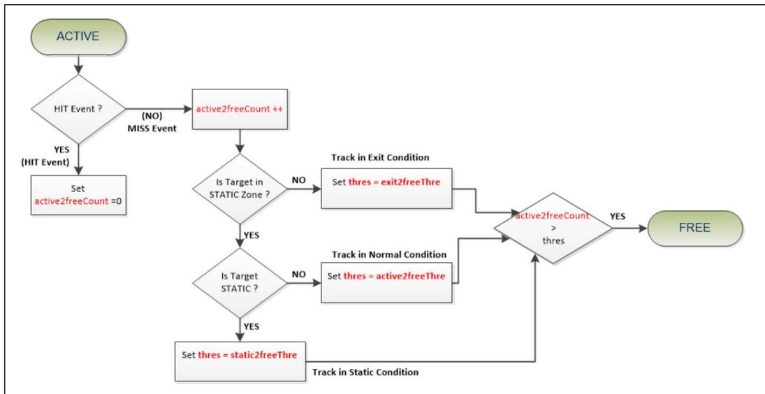
Figure 32. ACTIVE to FREE state transition flow diagram [53]
