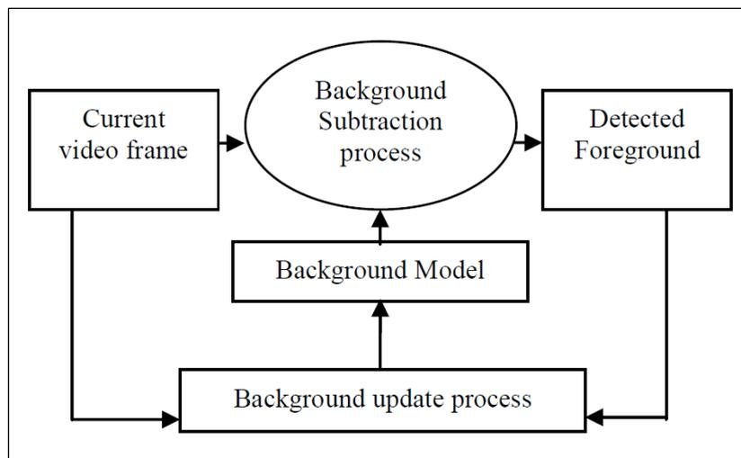
Figure 3. Block diagram of Background Subtraction process [11]
