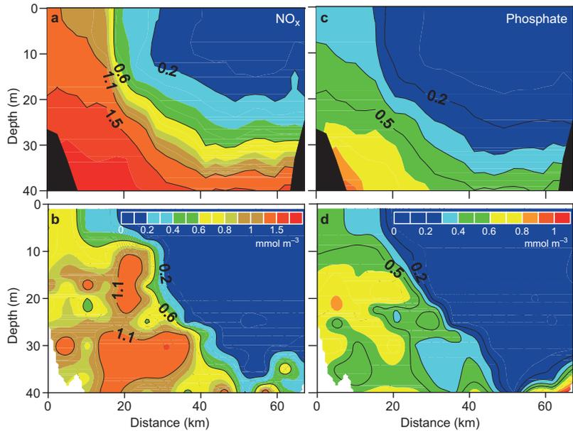
**Fig. 7.** Comparison of (a, c) simulated and (b, d) measured  $\text{NO}_x$  and  $\text{PO}_4$  concentrations along the transect between Tallinn and Helsinki on 8 August. The values on the x-axis denote the distance from the southernmost sampling station. Separate colour scales for  $\text{NO}_x$  and  $\text{PO}_4$  concentrations were used.
