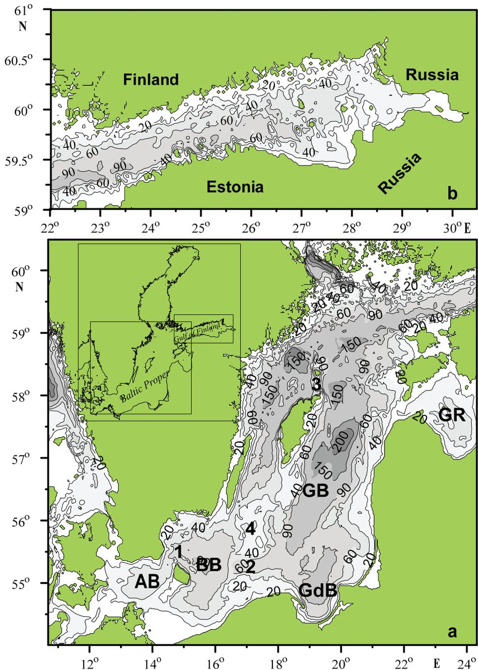
Figure 1: Bathymetric maps of the BP (a) and the GoF (b). The abbreviations on (a) mark the following sea basins: (AB) Arkona Basin; (BB) Bornholm Basin; (GdB) Gulf of Gdansk; (GB) Gotland Basin; (GR) Gulf of Riga. Digits on (a) mark 1 – Bornholm Channel, 2– Slupsk Furrow, 3 – Fårö channel, 4 – Hoburg-Midsjö Bank
