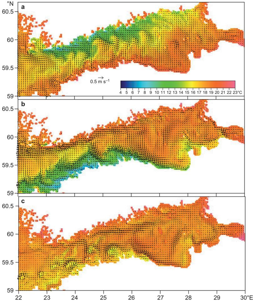
**Fig. 4.** Simulated surface layer currents (vectors) and SST in the Gulf in the course of upwelling/downwelling events on (a) 26 July (01:00 UTC), (b) 13 August (17:00 UTC), and (c) 19 August (18:15 UTC). The vectors of current are depicted in every fourth grid nodes.
