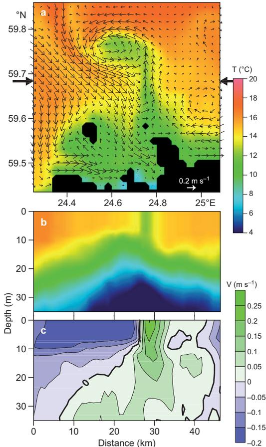
**Fig. 6.** Snapshot of a simulated cold-water filament and related transverse squirt transforming into a cyclonic eddy. (a) SST and surface layer currents off Tallinn Bay on 17 August, 06:45 UTC, (b) temperature, and (c)  $v$  component of velocity vs. distance and depth on a zonal transect marked by thick arrows. Velocity vectors are depicted in every second grid nodes.
