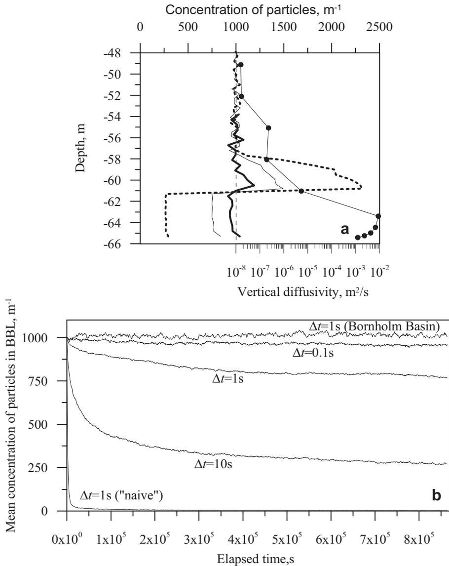
Figure 4: The theoretical validation of random walk model (a): The depth profiles of the particle concentration at the instant  $t=10$  days obtained from the random walk model in the course of testing experiments with the vertically homogenous initial distribution of the particles at different values of time increment  $\Delta t$ . (b): The time dependence of the mean particle concentration in the BBL found from testing experiments at different  $\Delta t$
