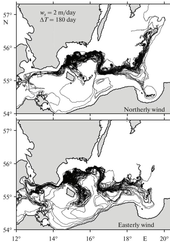
**Fig. 6.** The pathways of particles with the settling velocity  $w_s = 2$  m/day released in the bottom layer of the Bornholm strait at northerly and southerly winds. Here and in what follows, the grey crosses mark the site of the particle release and  $\Delta T$  designates the period of the particle walking.
