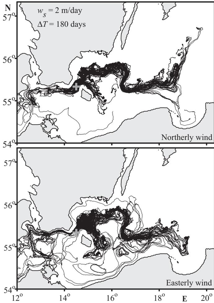
Figure 8: The pathways of particles with the settling velocity  $w_s = 2$  m/day released in the BBL of the Bornholm Strait at northerly and easterly winds
