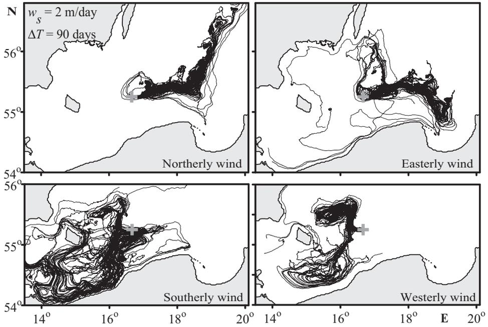
Figure 10: The pathways of suspended particles released in the bottom layer of the Slupsk Furrow under winds of different conditions
