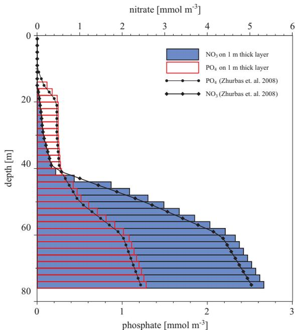
**Figure 3.** The initial nutrient concentration of different layers at  $59^{\circ}37.5'N$ ,  $23^{\circ}46'E$  compared with the profiles based on measurements performed onboard r/v 'Aranda' on 20 July 1999 (Zhurbas et al. 2008)
