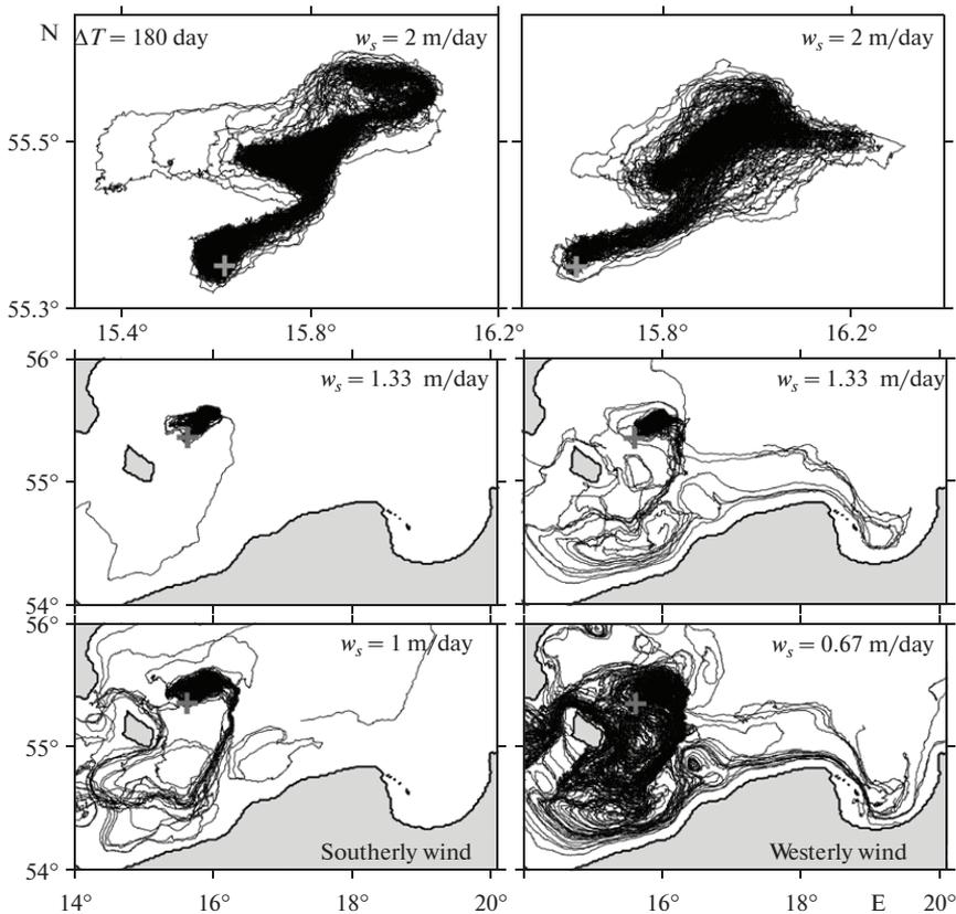
Fig. 9. Pathways of particles characterized by different settling velocities  $w_s$  and released in the bottom layer of the Bornholm Basin under the southerly (on the left) and westerly (on the right) winds. The scale in upper panel is increased in the proportion 20 : 3.
