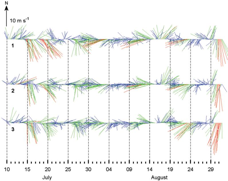
**Fig. 2.** Time series of the 10-m level HIRLAM wind vector in the (1) western, (2) central and (3) eastern parts of the Gulf of Finland for the period 10 July–31 August, 2006. Colours: blue = wind speed < 6 m s<sup>-1</sup>, green = 6 ≤ wind speed ≤ 10 m s<sup>-1</sup>, red = wind speed > 10 m s<sup>-1</sup>.
