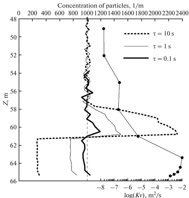
Fig. 3. The depth profiles of the particle concentration at the instant  $t = 10$  days obtained from the walking model (6) in the course of testing experiments with the vertically homogenous initial distribution of the particles at different values of the time increment  $\tau$ . The right-hand part of the picture shows the bottom sector of the depth profile of  $Kv$  at the Slupsk Sill used in the testing experiments.
