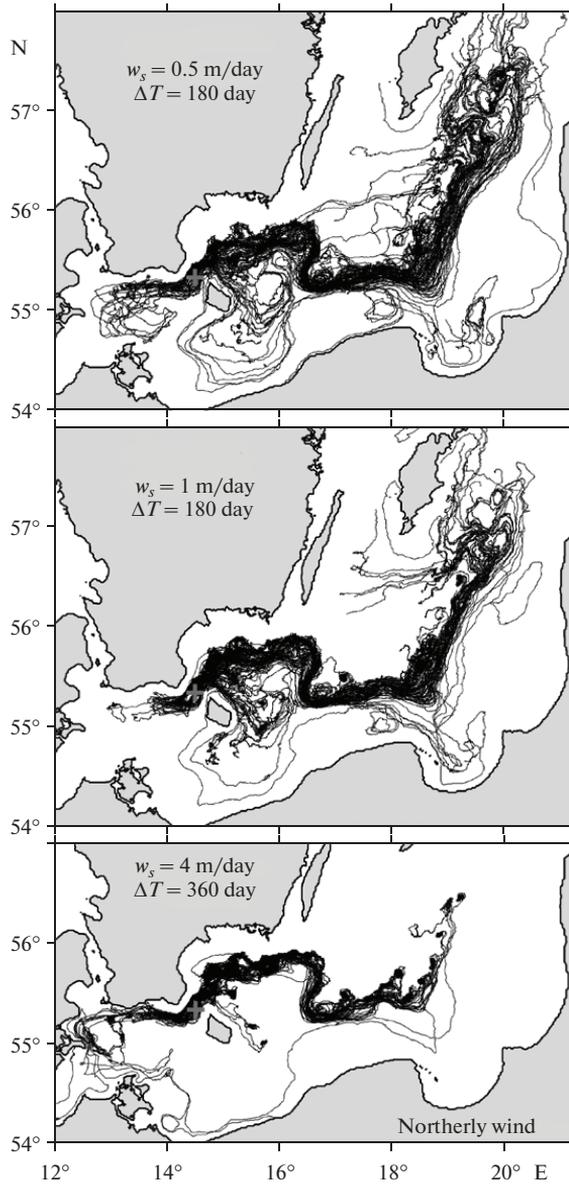
Fig. 7. Pathways of particles characterized by different settling velocities  $w_s$  and released in the bottom layer of the Bornholm Basin under a northerly wind.
