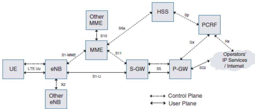
Figure 3. EPC detailed level architecture [7]
