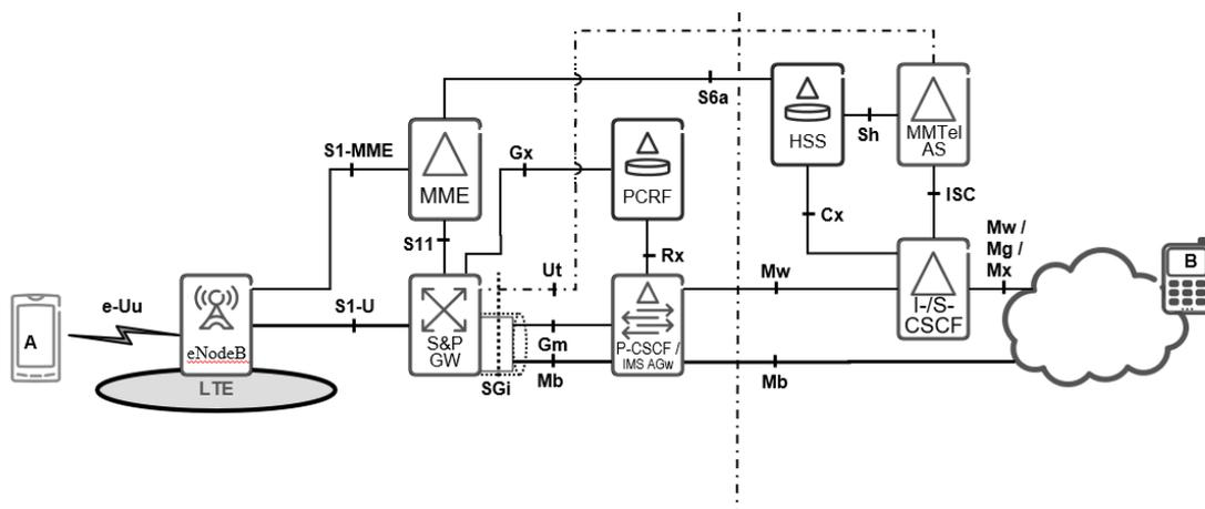
Figure 9. IMS architecture interfaced to EPC. [7]
