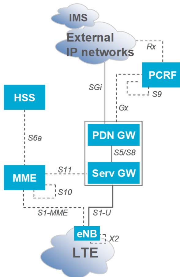
Figure 5. EPC main control plane and user plane interfaces. [7]
