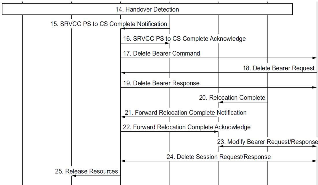
Figure 20. SRVCC Handover completion. [7]
