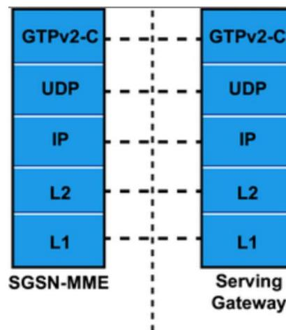
Figure 6. S11 interface protocol stack. [7]
