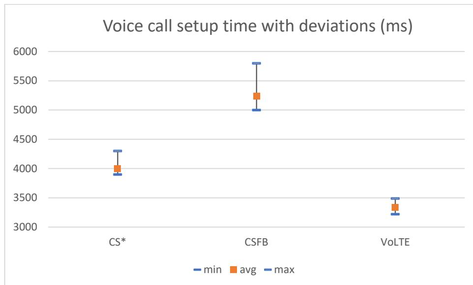
Figure 24. Voice call setup delay times. CS\* is estimated value.
