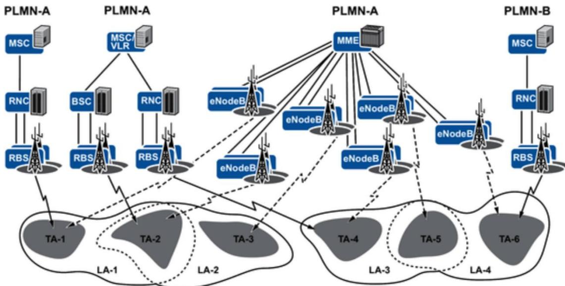
Figure 13. TA-LA mapping example [7]
