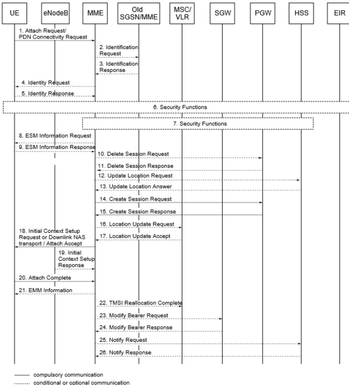
Figure 8. Terminal initial attach procedure in EPC network. [7]
