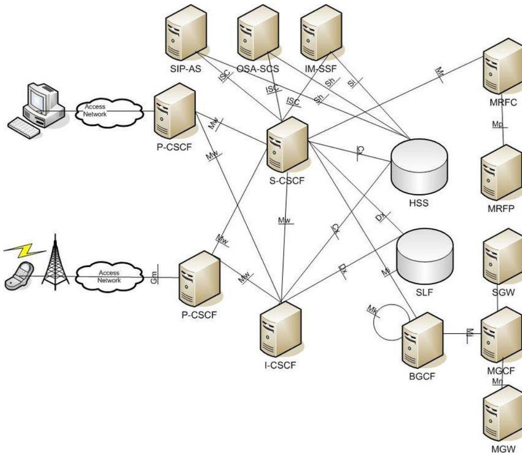
Figure 10. IMS core detailed architecture[14]
