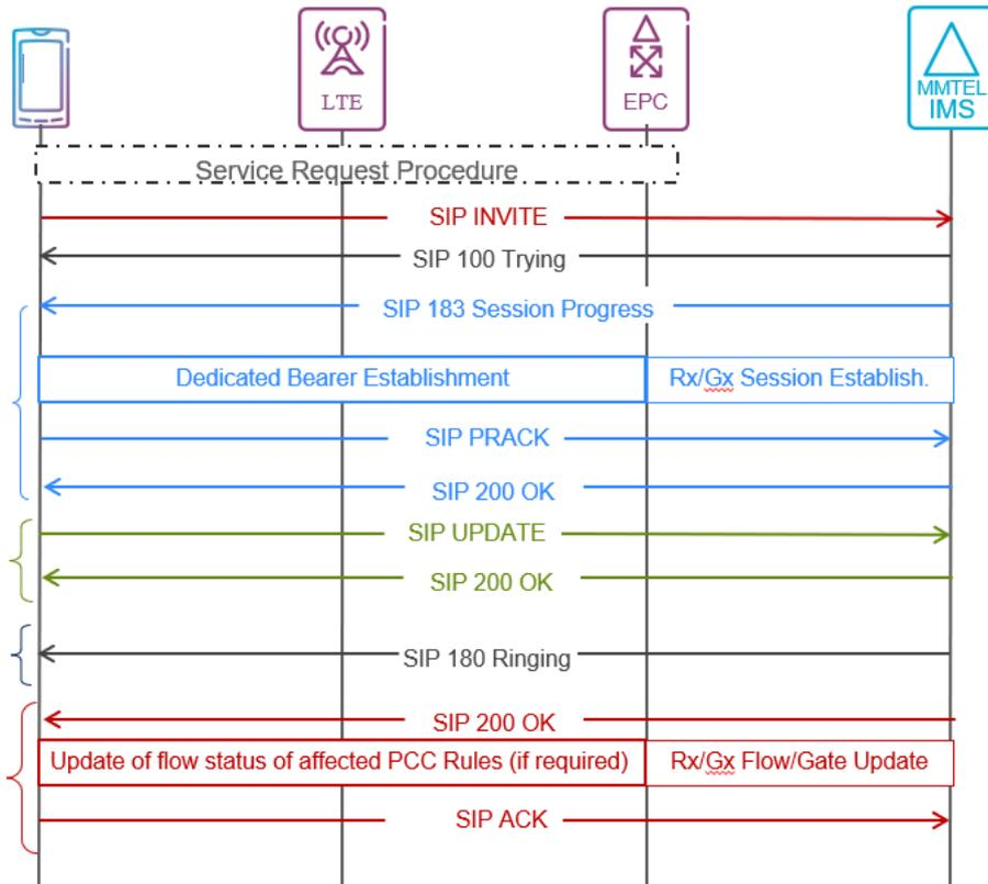
Figure 22. VoLTE call originating call flow. [7]
