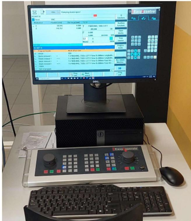
Figure 2.14. Turning machine controlling computer
