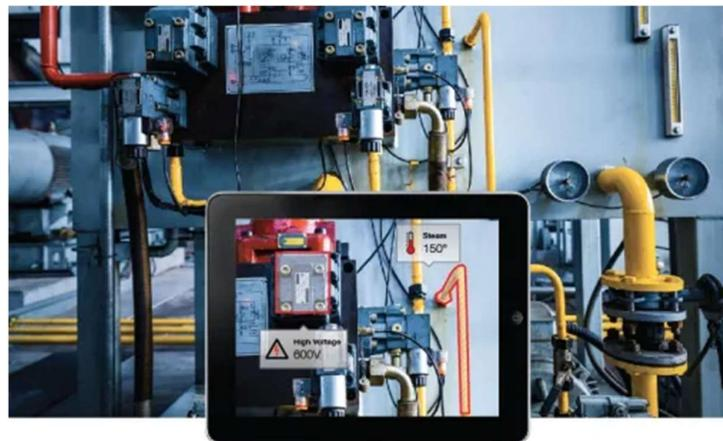
Figure 2.6. Augmented Reality maintenance screen. The digital data is aligned with the real world elements [13].
