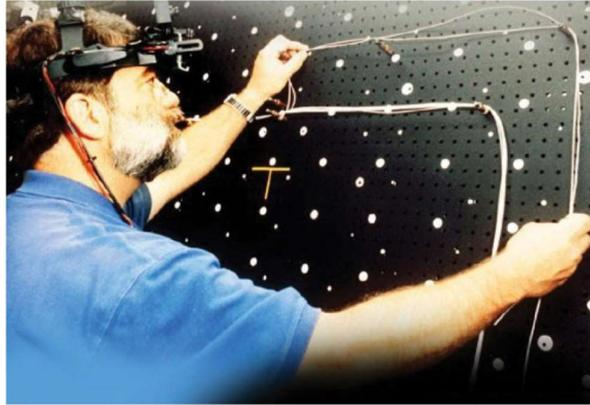
Figure 2.5. Researchers at Boeing looking through HMD guiding the assembly of wire bundles [12]
