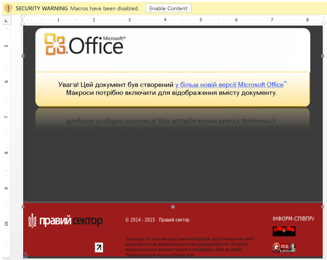
Figure 3. Malicious Microsoft Office document used in 2015 Ukrainian power-grid cyber-attack [101] As seen above, the attachment was in Ukrainian language to look more legitimate to employees of the electric companies. This is an important information and a takeaway
