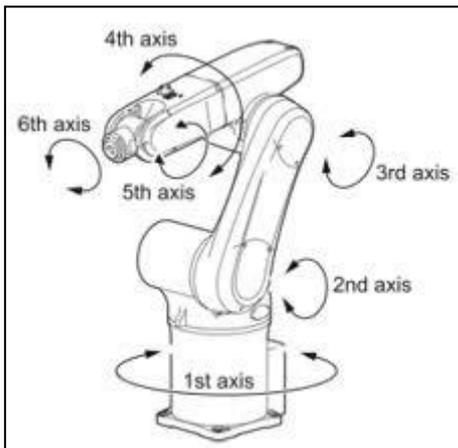
**Figure 6.** Scheme of 6-axis robot
