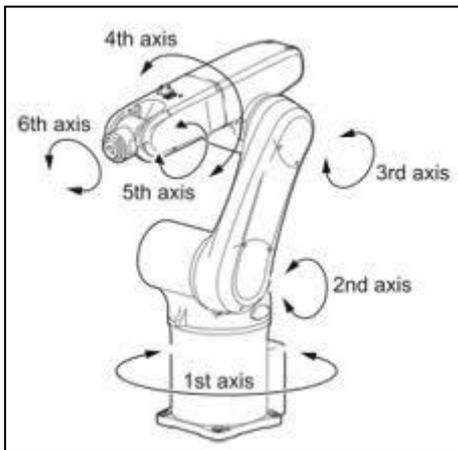
**Figure 6.** Scheme of 6-axis robot
