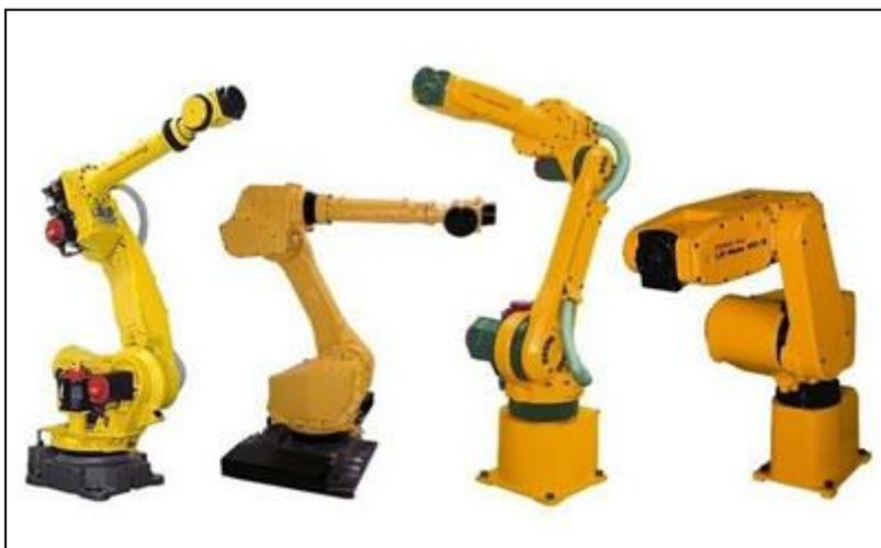
**Figure 7.** Real pictures of 6-axis robots
