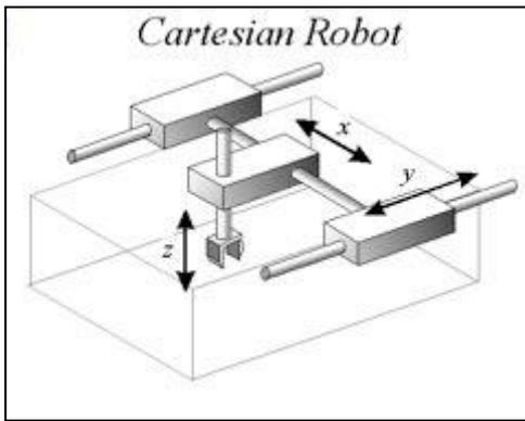
**Figure 2.** Plan of Cartesian robot
