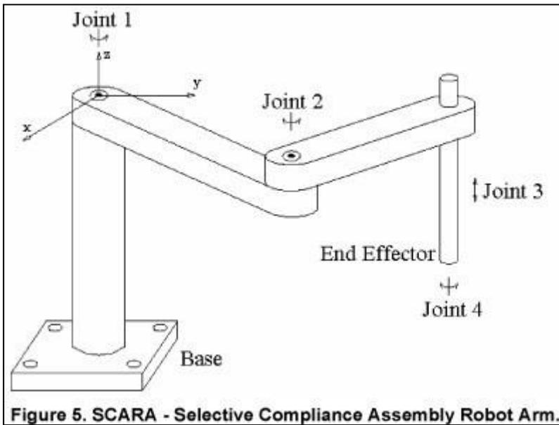
**Figure 4.** Plan of SCARA robot
