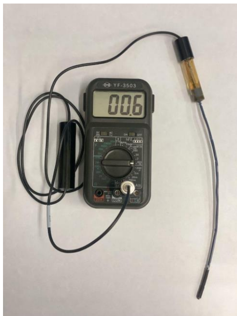
Figure 6. YFE-3505 multimeter and pH electrode (Ag/AgCl).
