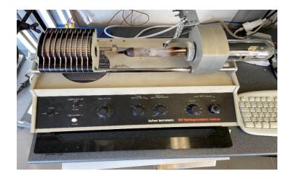
Figure 3.1 DuPont instruments 951 thermogravimetric analyzer
