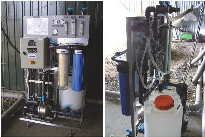
Figure 5.2. Experimental set-up of RO and NF (views from front and rear)
