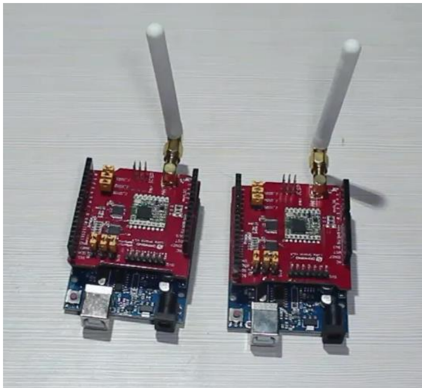
Figure 4.3. Attached pair of LoRa and Arduino board which acts as a server and client [38]
