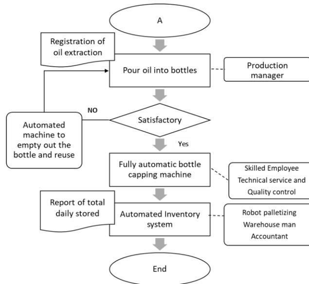
Figure 11 Diagram of oil manufacturing process II (redesigned)
