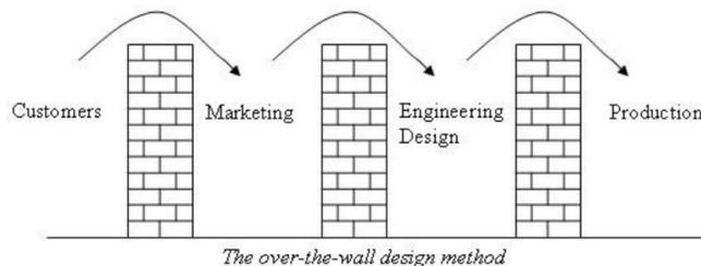
Figure 7 the over-the-wall design [26]
