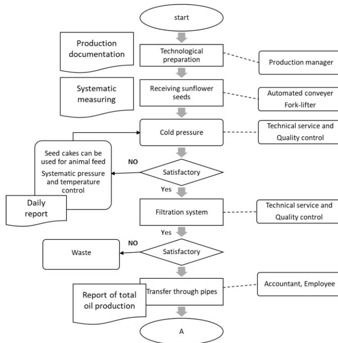
Figure 10 Diagram of oil manufacturing process I (redesigned)
