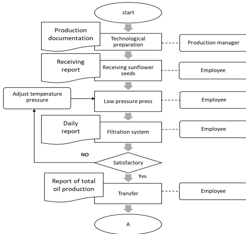
Figure 3 Diagram of oil flower manufacturing process in NAZGOL company I
