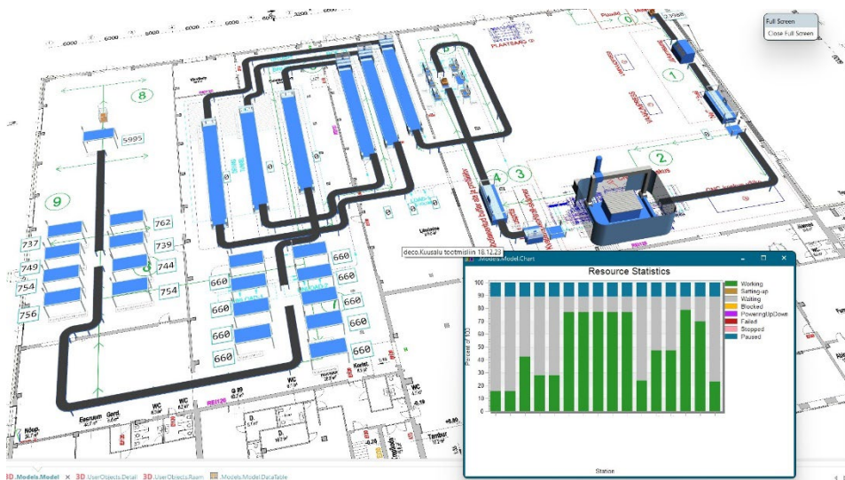
Figure 22. Virtual factory model of a wood industry production line in Siemens Plant Simulation, including resource statistics used for analyzing workstation utilization and bottlenecks (adapted from Publication VII).
