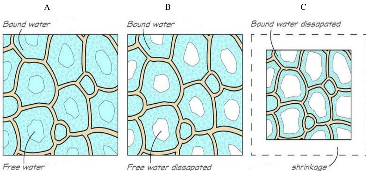
Figure 1.(A-B) water in the cell of green wood; (C) water in the cell of dry wood. Source: (Work Shop Companion. Google. 2009)
