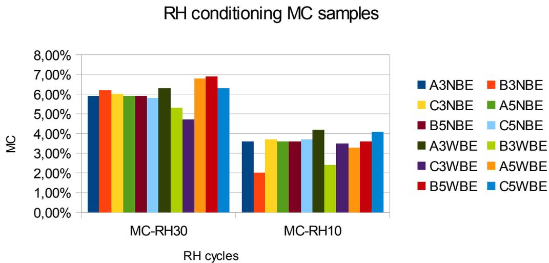
Figure 19. Chart of variation of MC for shorter cycle (from RH 30% to RH 10%)
