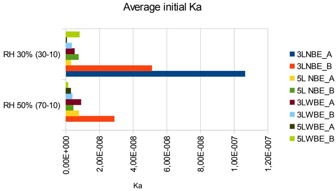
Figure 24. Chart Air Permeability coefficients  $k_a$  for all the panels in the initial conditions at RH 50% (cycle RH 70-10%) and RH 30%. (cycle RH 30-10%)
