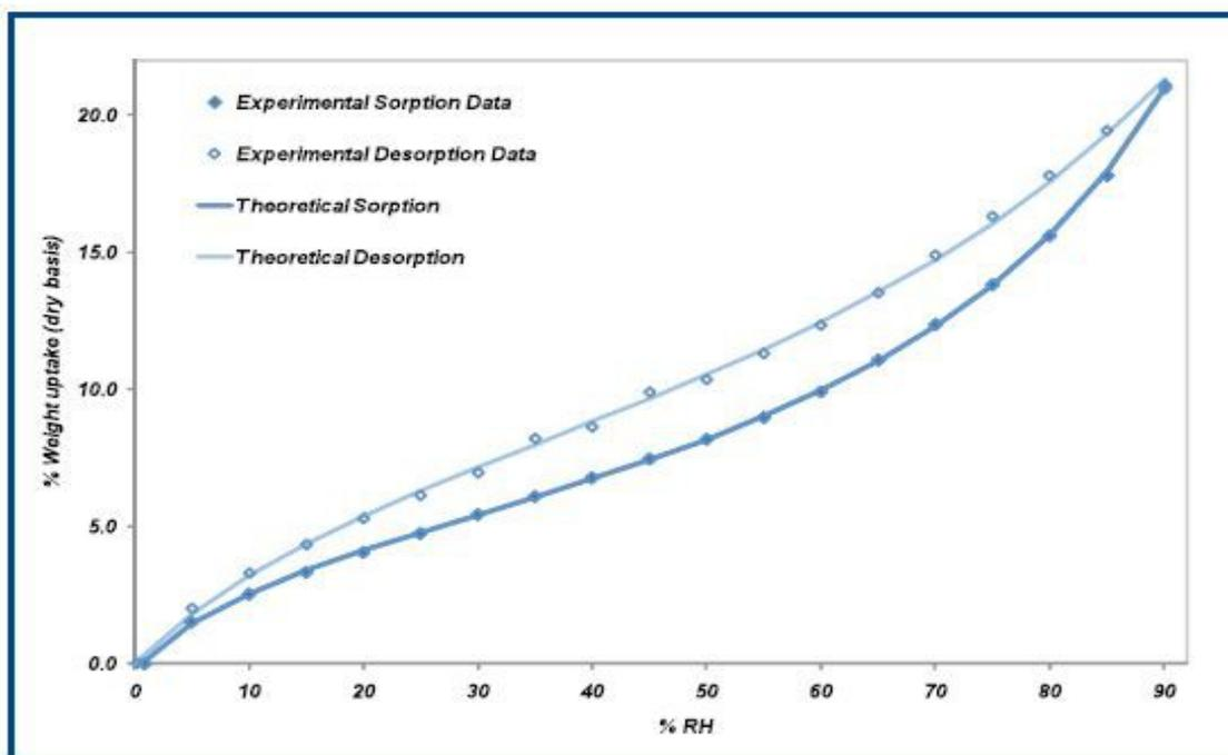
Figure 2. Classical Sorption-Desorption isotherm of wood. Source: (Azom. Google. 2015)
