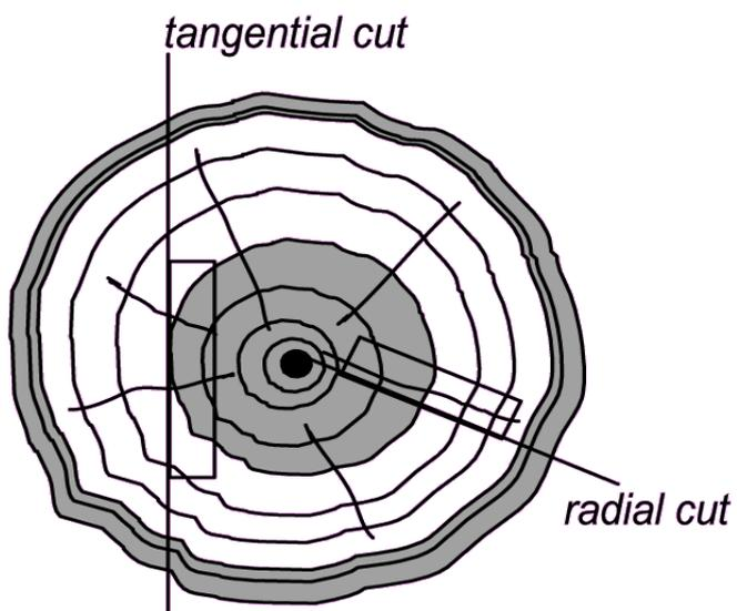
Figure 5. The risk of checking is greatest in timber where the heartwood reaches the surface (on the left). Source: (Geoff's woodwork. Google. 2016)
