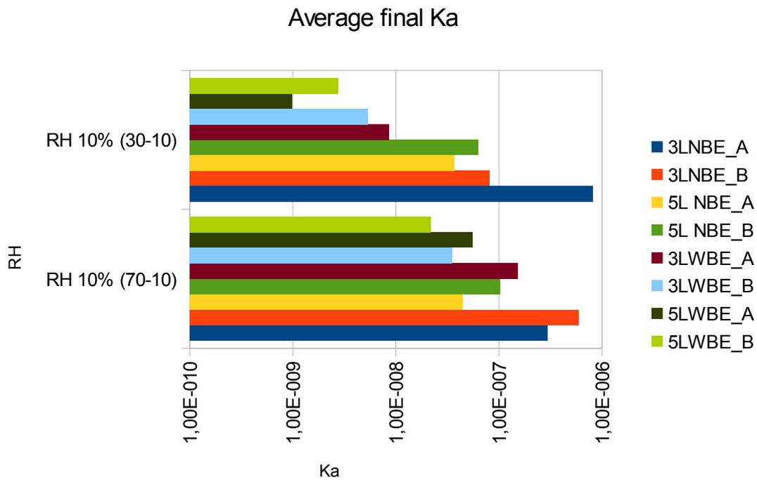
Figure 25. Chart Air Permeability coefficients  $k_a$  for all the panels in the final conditions at RH 10% (cycle RH 70-10 and cycle RH 30-10).
