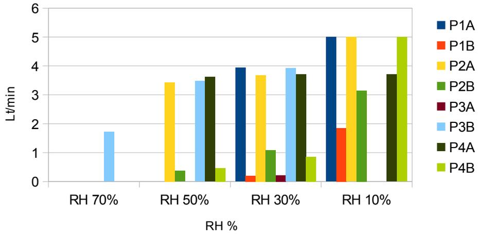
Max Air Leakage 5L NBE RH30%-10%
