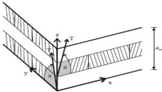
Figure 9. Definition of annual ring angle. Source: (Gereke T. and Niemz P., 2009)
