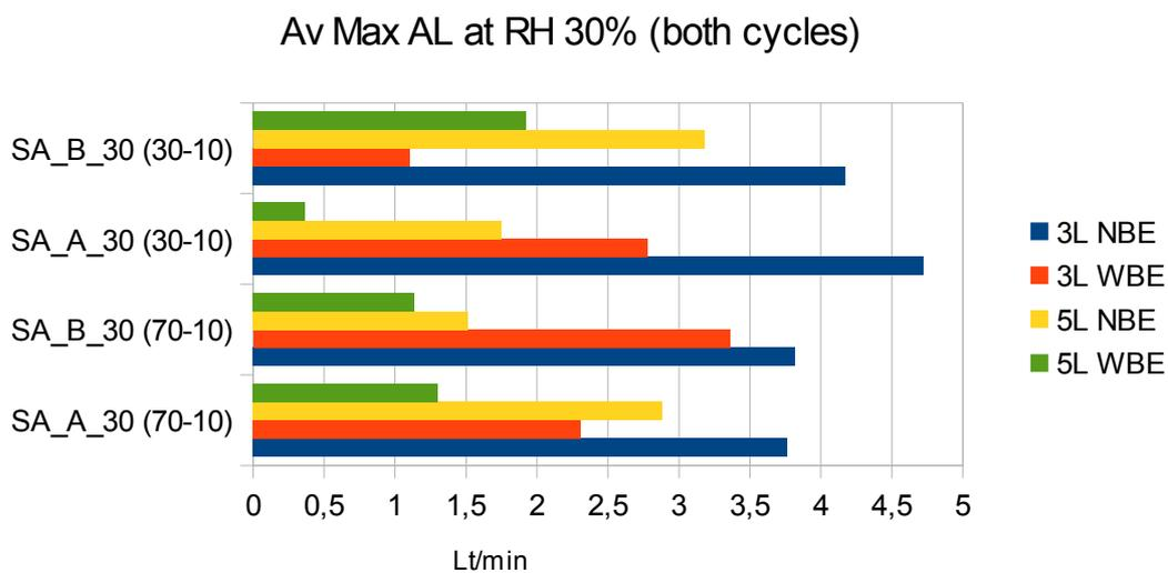
Figure 22. Chart RH-average maximum Air Flow for panels (24 panels) at RH 30% (cycle RH 70-10% and cycle RH 30-10%)
