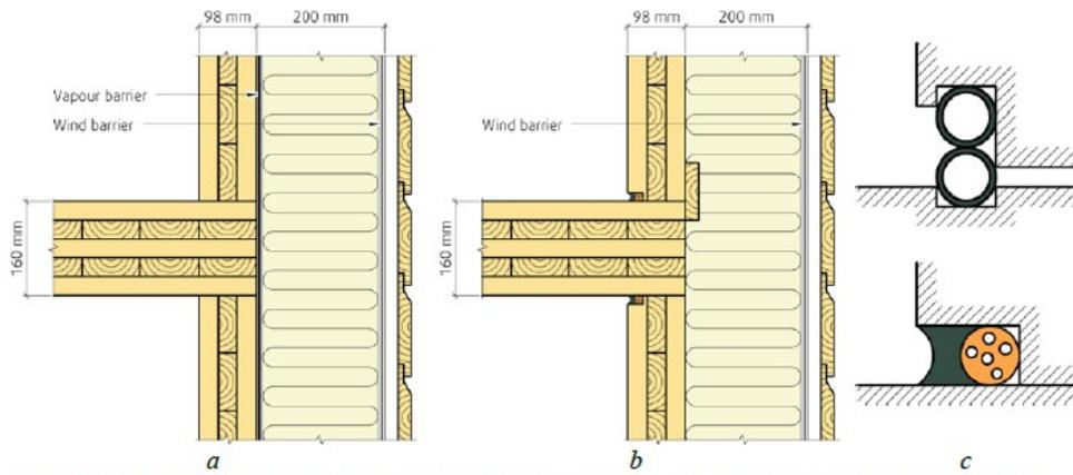
FIG 10. Cross section of CLT construction with separate water vapor barrier and wind barrier (a), and local sealing of joints between floor and wall elements with separate wind barrier under a ventilated wooden cladding (b). Examples of local sealing with rubber molding or sealing compound.
