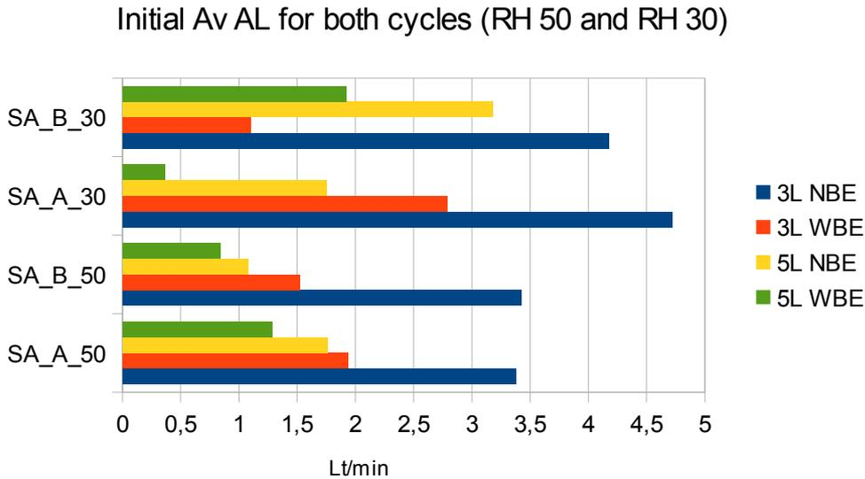
Figure 21. Chart RH-average maximum initial Air Flow (Lt/min) for panels (12 panels) at RH 50% (cycle RH 70-10%) and panels (12 panels) at RH 30% (cycle RH 30-10%)
