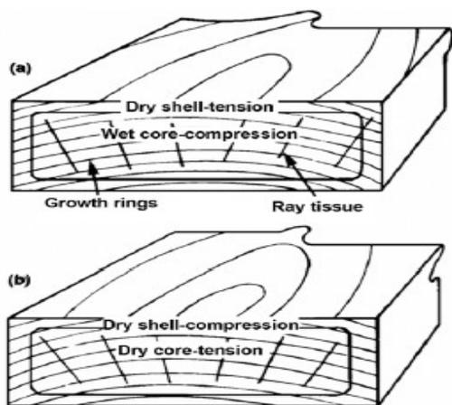
Figure 7. Development of drying stresses a) early b) later. Source: (Wood handbook USA. 2010)
