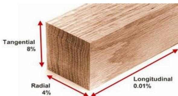
Figure 3. Shrinkage/swelling in wood for radial, tangential and longitudinal directions. Source: (Work Shop Companion. Google. 2009).
