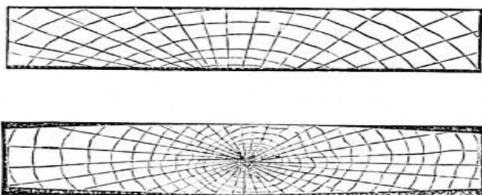
Figure 6. If the pitch is located within the cross section (bottom), most probably checks will occur. Source: (Wikisource. Google. 2016)
