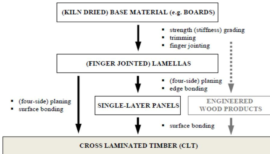
Figure 17. CLT process overview. Source: (Brandner R. *et al.*, *Sciencedirect*. 2014)
