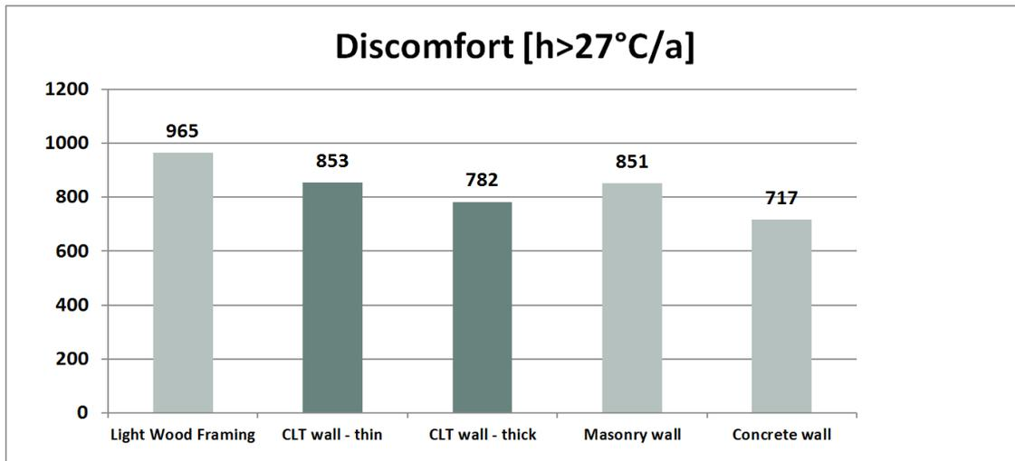
Figure 16. Thermal inertia of CLT in comparison to other building materials such as masonry or concrete. Source: (clt.info. 2015)
