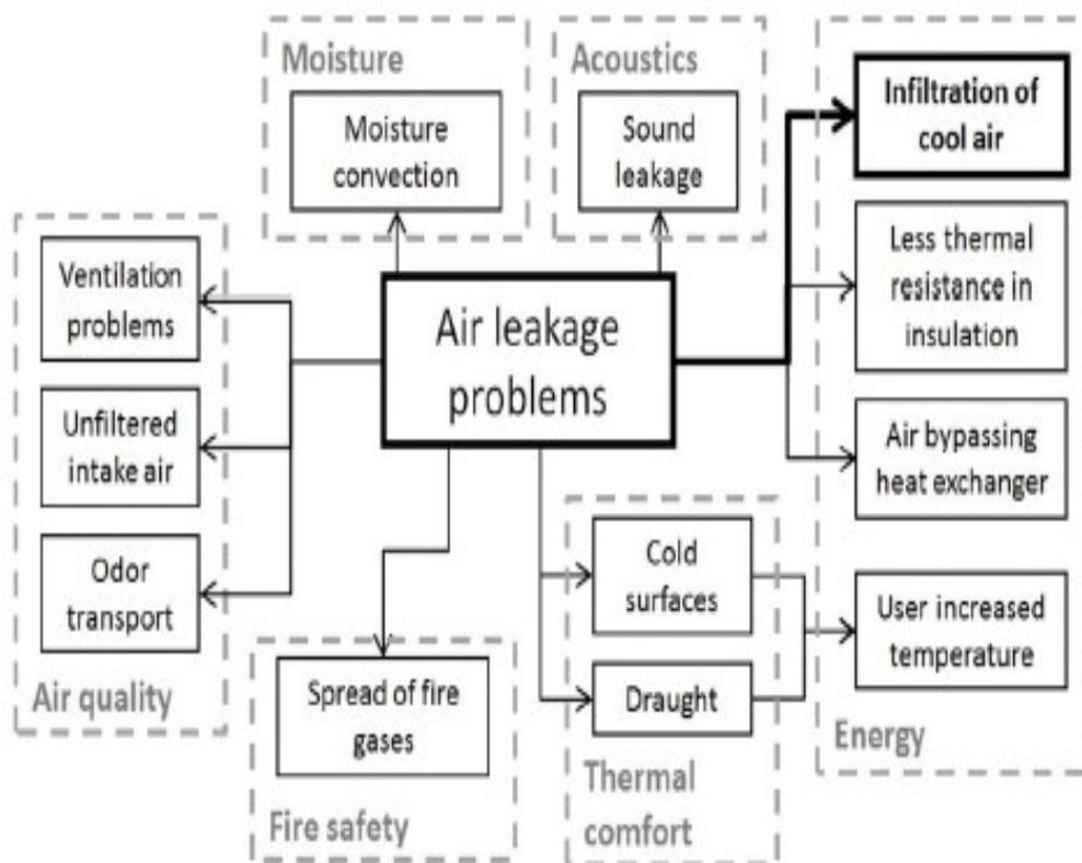
Figure 12. Problems related to air-leakage. Source: (Axel Berge. Google. 2013)
