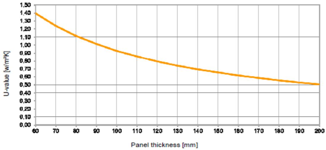
Figure 14. Variation of U-value through the thickness of clt panel. Source: (clt.info. 2015)
