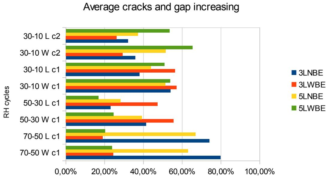
Figure 20. Chart of average increasing percentage of cracks and gaps increasing for all the panels, from RH 70% to RH 50% , from RH 50% to RH 30% (c1) and from RH 30% to RH 10% (c2), (W width, L length)
