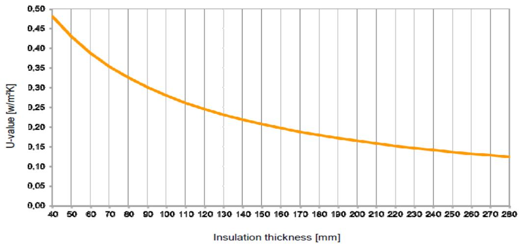
Figure 15. Variation of U-value through the thickness of the insulation (WLG 040 insulation material). Source: (clt.info. 2015)
