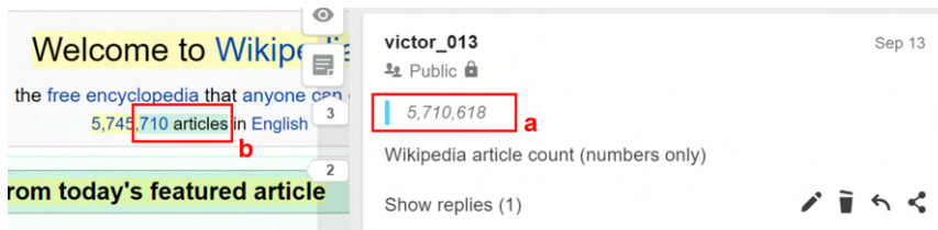
Figure 10 – Illustration of Hypothesis reattaching annotation at incorrect location. We have that (a) indicates the actual annotated anchor text i.e., “5,710,618”, while (b) indicates the text to which the annotation has been reattached (i.e., “710 articles”). Here, the position shift is caused by fuzzy string matching, as the algorithm finds that “5,710,618” matches more with “710 articles”, and not “5,745,710”. [publication II].
