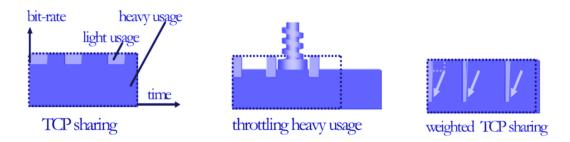
Figure 6 - Resource sharing. Left: TCP sharing (base case). Middle: Limit volume (DPI). Right:
