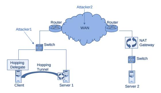
Figure 7 - Two designs for implementing port and address hopping (Recreated) [67]
