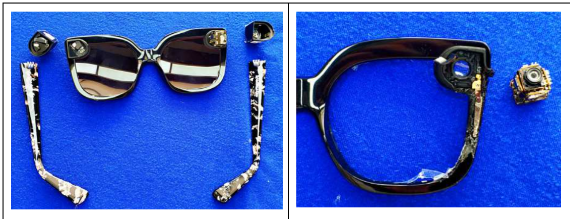
Figure 3. Snapchat Spectacles version 2 teardown - Sunglasses and camera [146][147]
