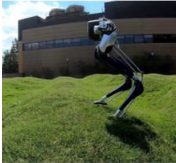
Figure 2.5: Cassie Robot Dynamically and Statically Balanced on Rough Terrain [4]
