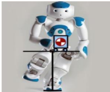
Figure 2.13: Robot NAO is an example of cart-table model [14]
