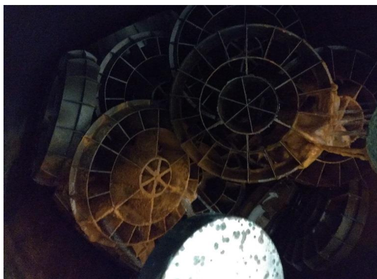
Figure 3.1 MBBR carriers during the operation in aerator
