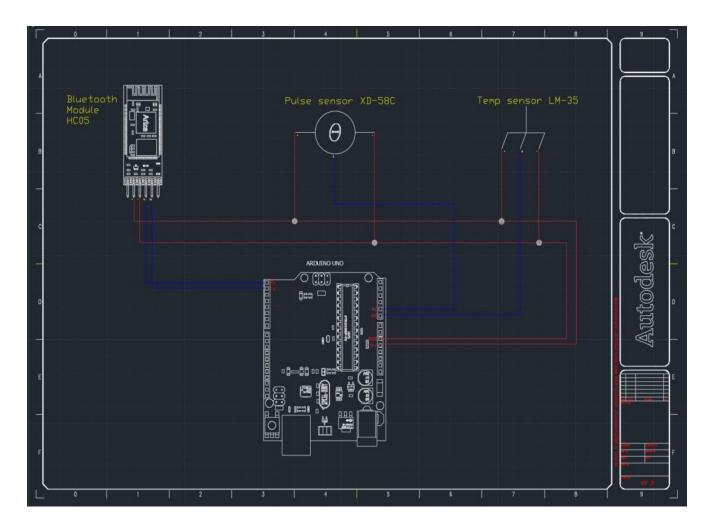
Figure 9: Overall Hardware Design
