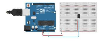
Figure 7. Temperature Sensor LM35
