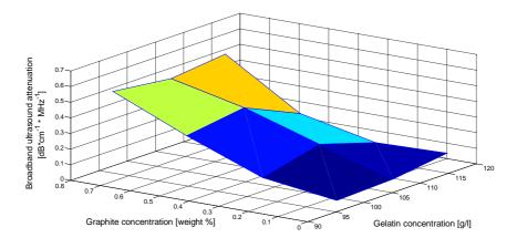
Figure 1.5 Broadband US attenuation in respect to gelatin and graphite concentrations
