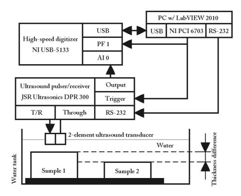
Figure 1.2 US attenuation measuring setup (image adapted from [42])
