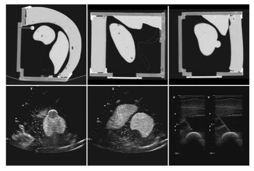
Figure 2.8 Kidney box phantom CT scan (upper row) and US images (lower row: left - visibility of the kidney and tumor with 4C probe; middle - visible kidney and liver with 4C probe; right - needle visibility near the tumor with 10L probe)
