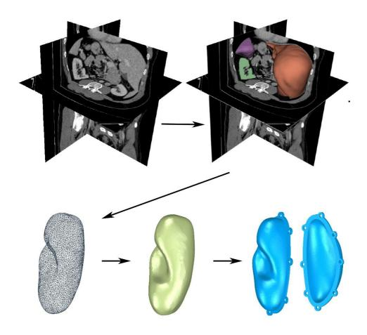
Figure 1.7 Organ reconstruction from CT scan (From left to right: (1) CT scan is opened in 3D Slicer software; (2) organs are segmented and models created; (3) models are saved as mesh in STereoLithography format; (4) organs are converted in native CAD format; (5) CAD software is used to create two or more-sided mold around the organ)
