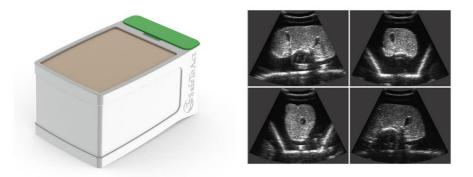
Figure 3.4 Commercial version of the kidney phantom and its US images
