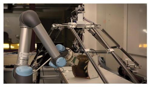
Figure 2.9 Kidney box phantom used in experimenting automated needle guidance with US probe handling done with UR5 robotic arm and needle guided with ISUR robot developed in ETH
