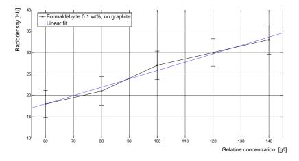
Figure 1.6 Gelatins mixture's radiodensity dependency on gelatin's concentration
