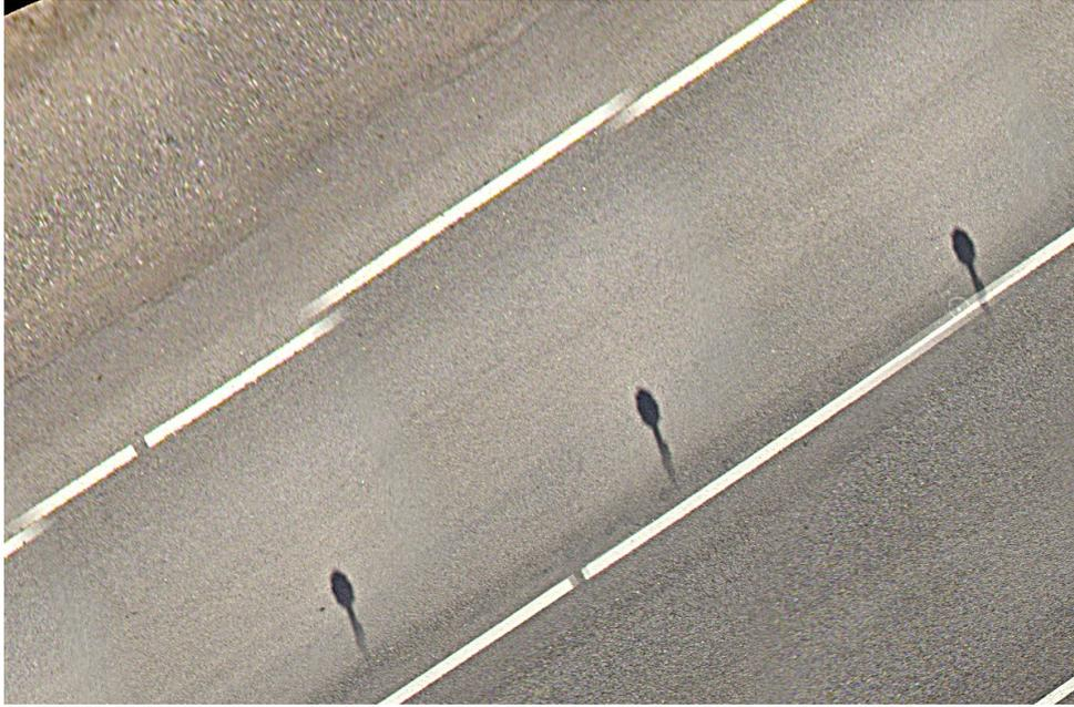
**Figure 4.** Persistent camera shadows and misaligned stitching from a generated orthophoto.
