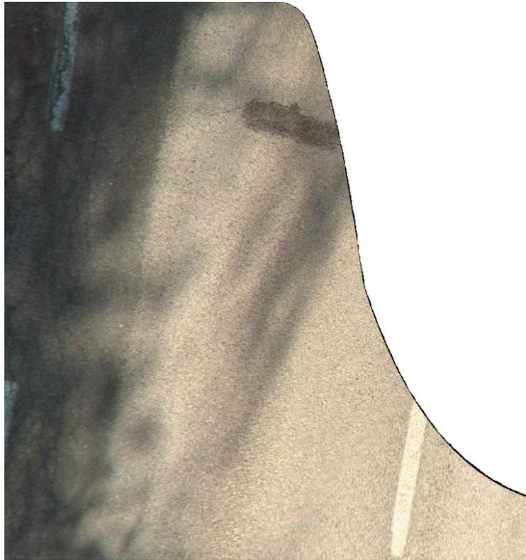
**Figure 6.** Difficult to assess part of the orthoframe belonging to test the set. The difficulties include shadows cast by trees, obfuscated alligator cracking on the left side of the road, inconsistent lighting, a dark patch and unclear road margins.
