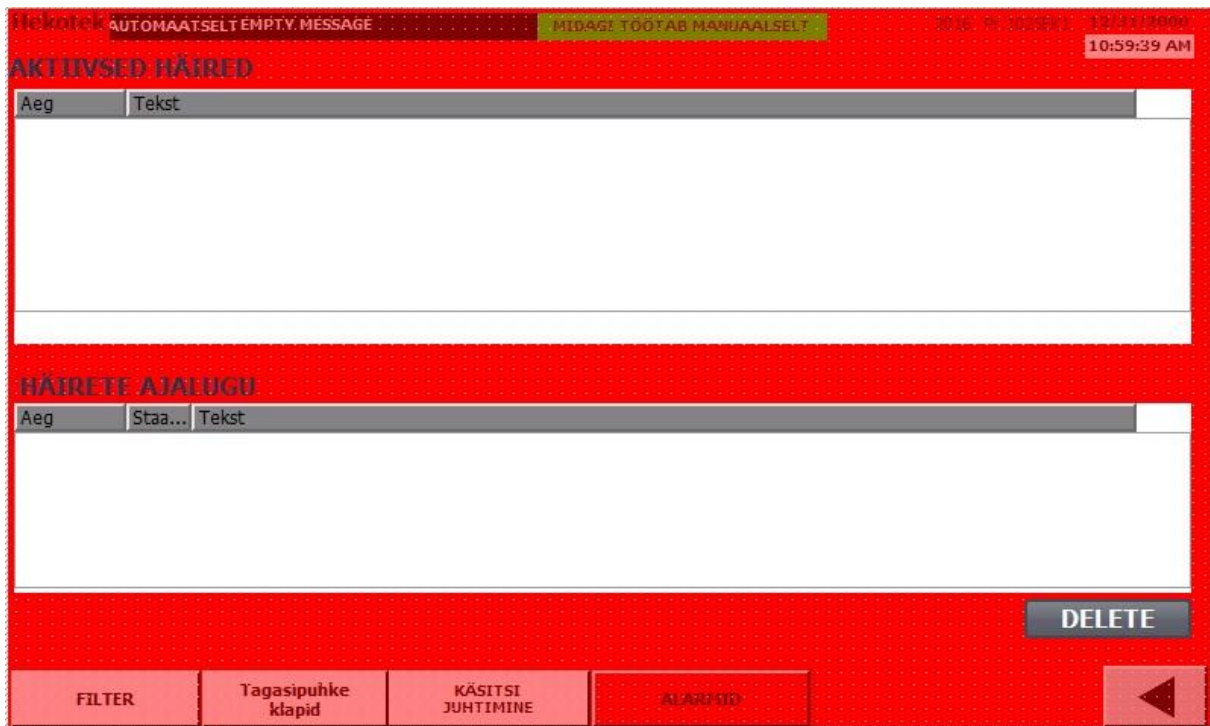
Figure 5.3 HMI alarms screen
