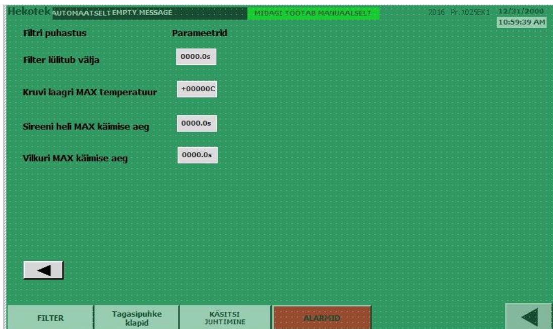
Figure 8.4 Filter cleaning settings control in HMI
