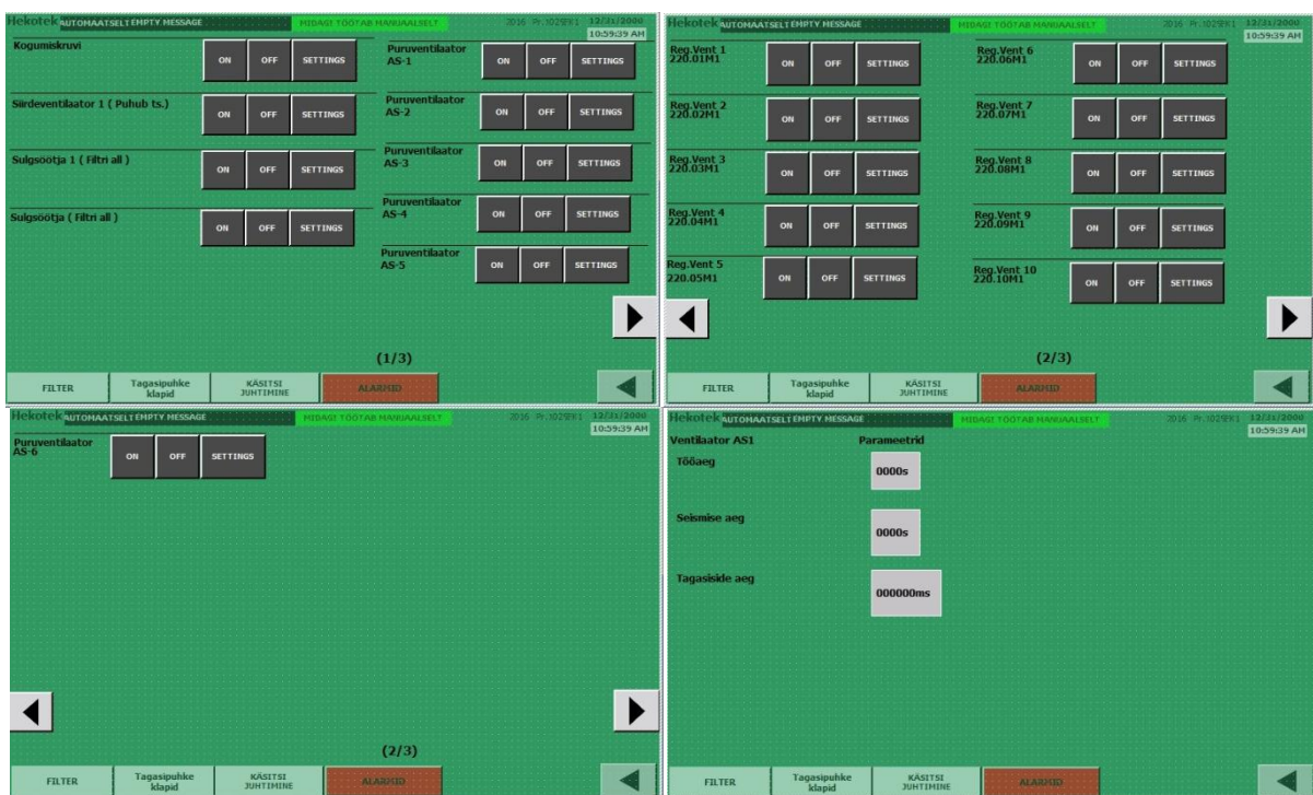
Figure 8.2 Filter motors manual control in HMI
