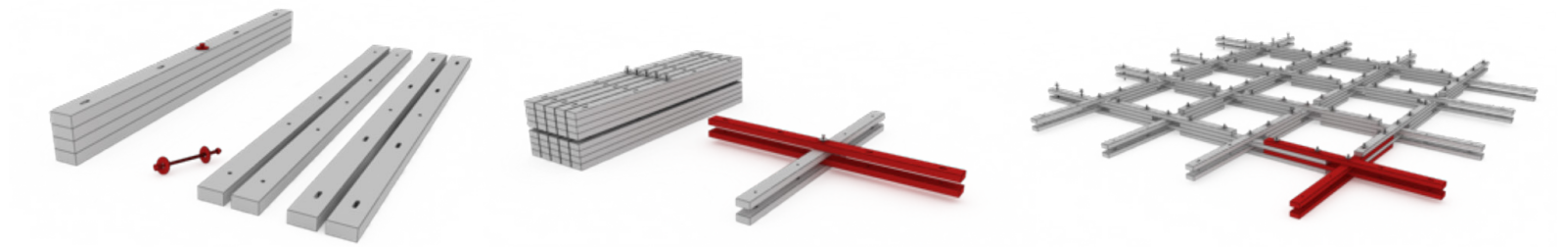
Figure 35. Segment laths. From module to assembly. Source: Dyvik, S.H., Mork, J.H., Nilsen, M. & Luczkowski, M. (2016)
