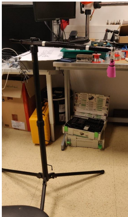
Figure 24. Ultrasonic distance sensor testing setup
