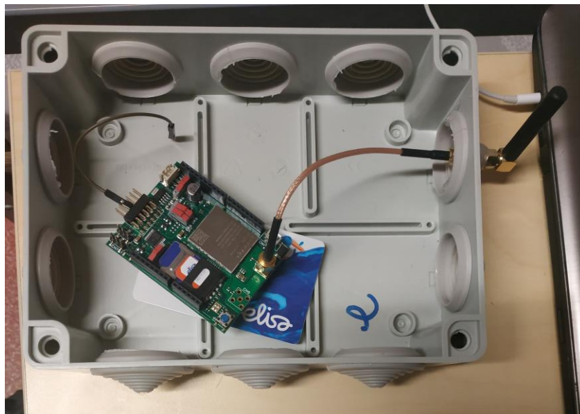
Figure 6. Avnet Silica NB-IoT BG96 (Quectel) shield with an NB-IoT SIM
