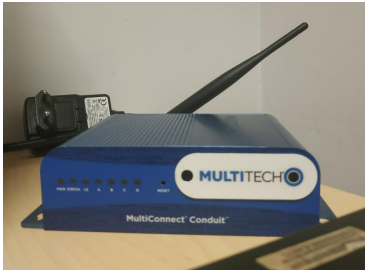
Figure 7. MultiTech Conduit MTCDDT 246L LoRa gateway
