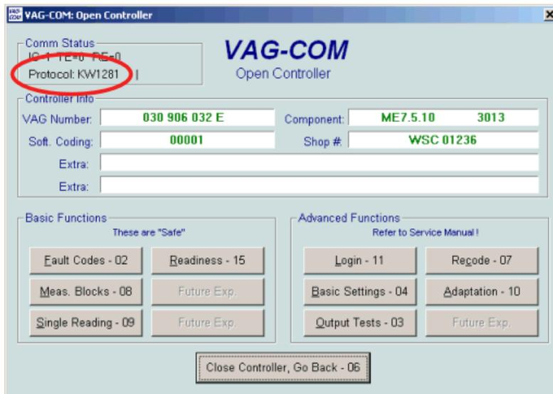
Figure 17. Checking what OBD2 protocol you ECU is using with VAG-COM. [28]
