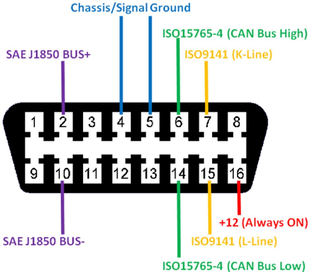
Figure 13. OBD-2 pinout with all default pins marked, the KW-1281 uses K-Line and also sometimes L-line. Also, every diagnostics device must always be connected to +12V and ground.
