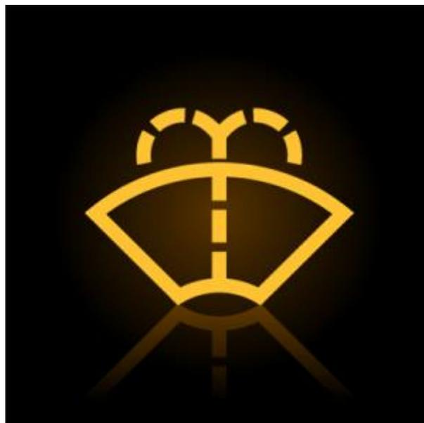
Figure 9. Low wiper fluid light. Sometimes this light is accompanied with a short alarm sound. [22]
