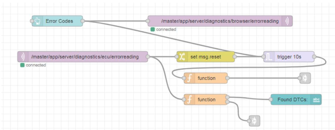
Figure 29. Send command to read error codes flow
