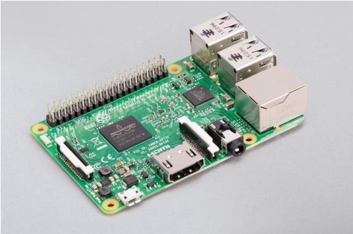
Figure 3. Raspberry Pi 3 model B [15]
