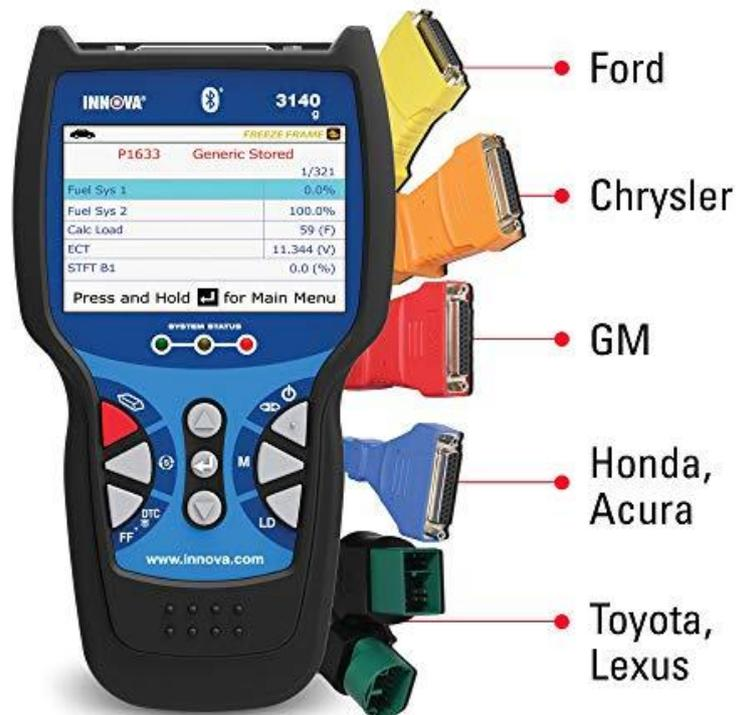
Figure 12. OBD-1 diagnostics tool which shows that different manufactures had different connection ports for diagnostics.
