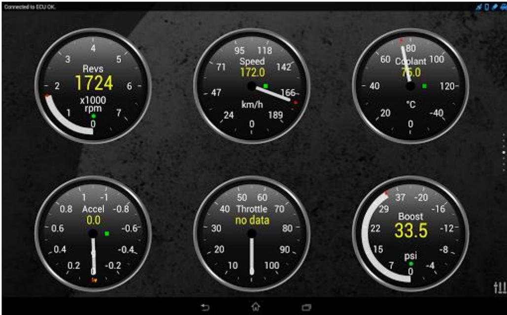
Figure 15. Screenshot of a mobile app called Torque. This app allows you to connect to your car with your phone using a Bluetooth OBD-2 diagnostics device. It sends data to your phone and the app displays the car's engine revolutions, car speed and coolant temperature. It can also be seen that the app failed to receive the throttle position. This could be because the diagnostics protocol the vehicle uses is not fully supported by the diagnostics device or the app itself.
