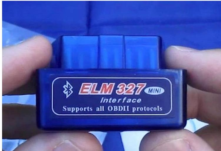
Figure 16. A very compact ELM device that is plugged into the vehicles OBD-2 socket and then connected to the phone with Bluetooth. This device can read data from most OBD-2 vehicles, but is missing the support for older vehicles.
