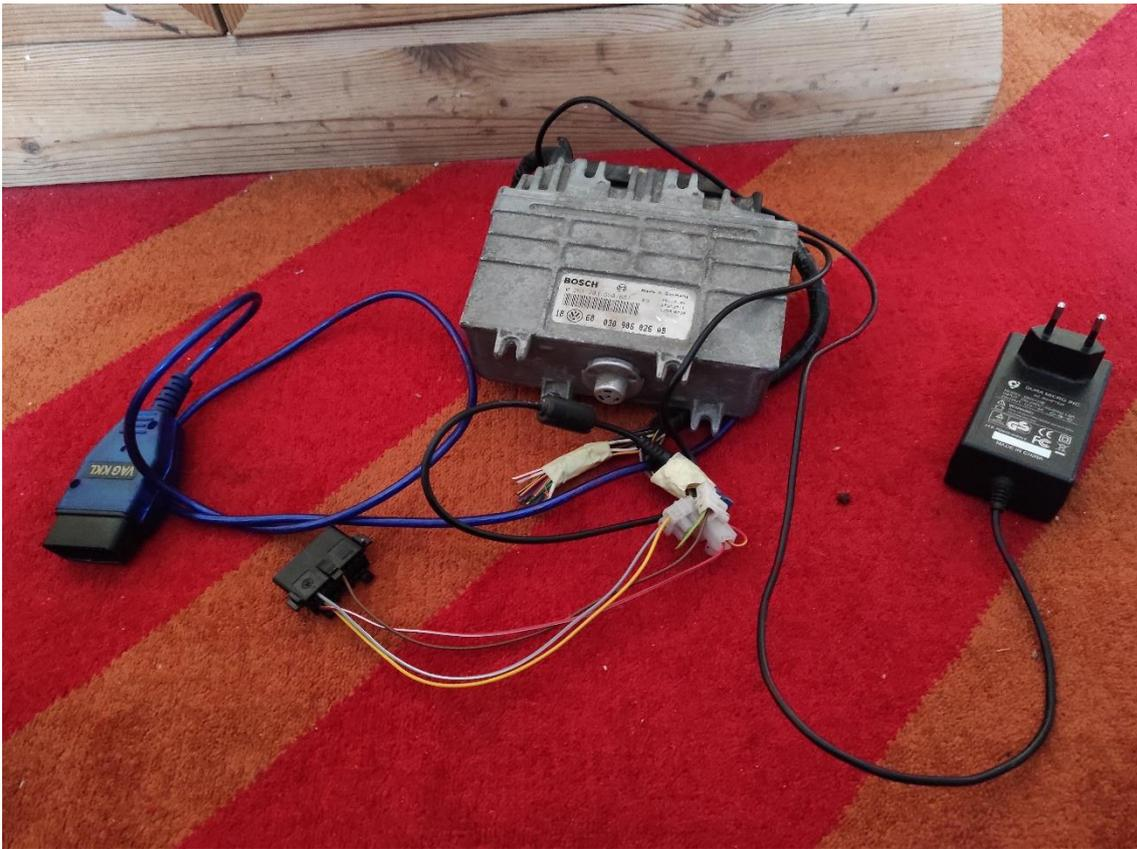
Figure 31. ECU with 12V adapter and OBD-2 cable
