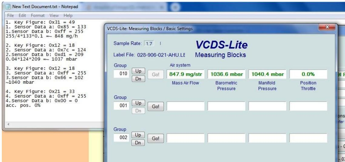
Figure 20. First test – engine running, read sensors in group 10
