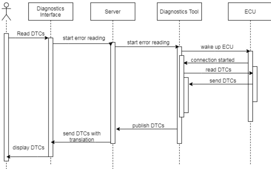
Figure 34. read DTCs algorithm
