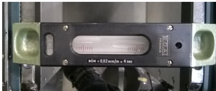
Figure 34: Spirit level in the jig
