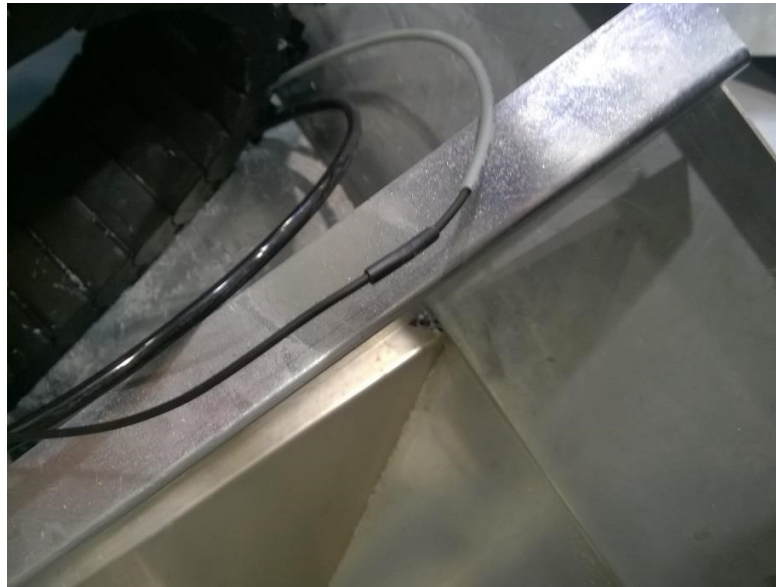
Figure 21: Fixing detail of two fiber cables
