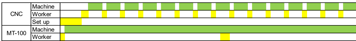
Figure 43: Worker interaction with machine in CNC and robot cell for a single batch
