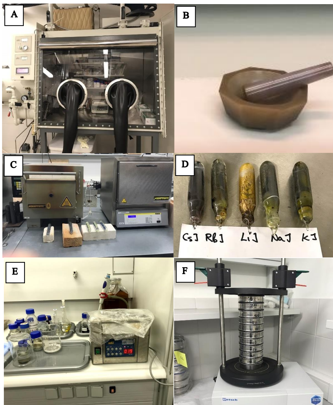
Figure 2.1 Experimental steps of the monograin powder preparation process: (A) glove box filled with Argon gas, (B) the precursors were mixed manually in agate mortar to ensure homogeneous mixture, (C) chamber furnace used for annealing, (D) annealed samples with different flux materials showing their different colors and appearances, (E) ultrasonic bath used during washing process to remove flux material, (F) the sieving machine containing sieves with different mesh widths (ranging from 38\mu\text{m} to 112\mu\text{m} ).
