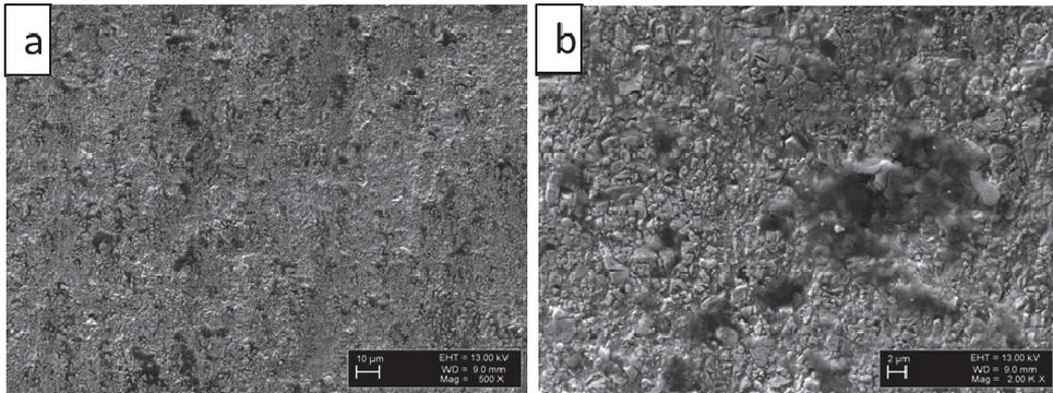
**Fig. 4:** Abrasive rubber-wheel wear of Z5 at magnification (a) 500X (b) 2000X
