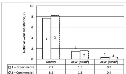
**Fig. 5.** Relative wear resistance of sprayed coatings to steel C45.
