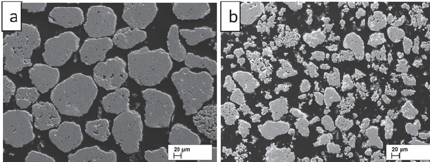
Fig. 2: Particle size and shape (a) before and (b) after disintegrator milling
