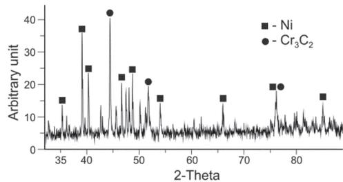
**Fig. 3.** XRD patterns of Cr<sub>3</sub>C<sub>2</sub>–20Ni powder produced by MATS.
