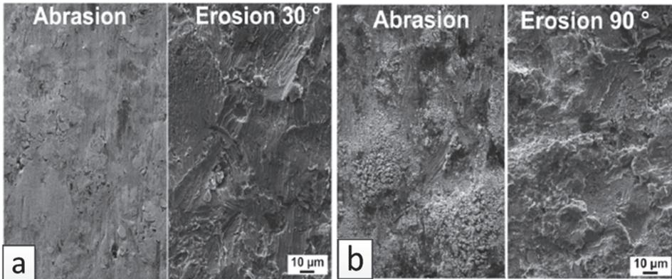
Figure 3.8 Topography of worn surfaces at ARWW and AEW of sprayed coatings based on self-fluxing alloy and consisting of MDM hardmetal/cermet hard phase: a –  $(Cr_3C_2-Ni) + FeCrSiB$ ; b –  $(WC-Co) + NiCrSiB$
