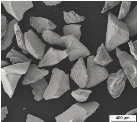
Figure 1.3 Micrograph of WC-15wt%Co hardmetal powder produced by disintegrator milling [Kulu, 2003]
