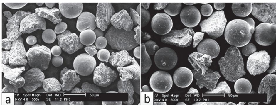
Figure 3.1 Morphology of self-fluxing alloy - MDM hard phase spray powders: a – (Cr<sub>3</sub>C<sub>2</sub>-Ni)+FeCrSiB; b – (WC-Co)+FeCrSiB [Paper III]
