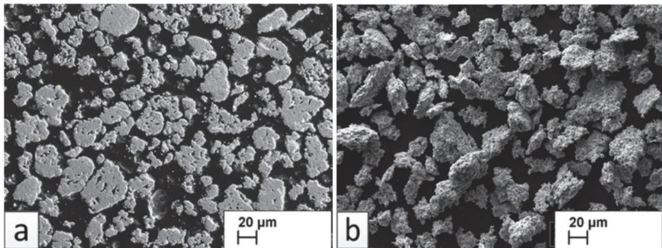
Figure 2.2 SEM images of spray powders: a – WC-Co; b – Cr<sub>3</sub>C<sub>2</sub>-Ni
