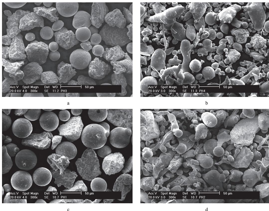
**Fig. 1.** Micrographs of composite spray powders: a – (Cr<sub>3</sub>C<sub>2</sub>-Ni)+FeCrSiB; b – (Cr<sub>3</sub>C<sub>2</sub>-Ni)+NiCrSiB, c – (WC-Co)+FeCrSiB, d – (WC-Co)+NiCrSiB
