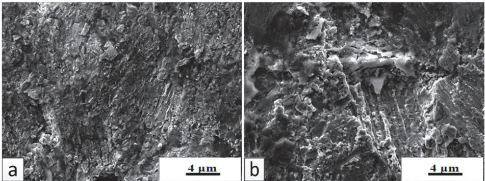
Figure 3.6 Topography of worn surfaces at AEW  $\alpha=30^\circ$ ) of sprayed coatings from MATS hardmetal/cermet powders: a – WC-Co; b – Cr<sub>3</sub>C<sub>2</sub>-Ni
