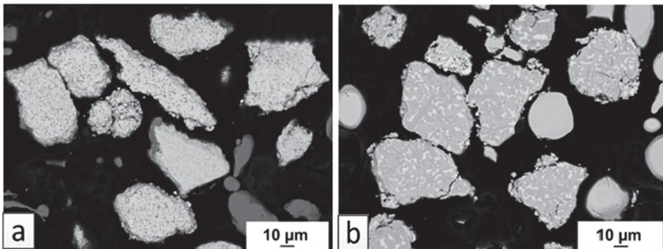
Figure 2.4 Cross-section micropolishes of disintegrator milled hardmetal/cermet powders: a – (WC-Co); b – (Cr<sub>3</sub>C<sub>2</sub>-Ni) [Paper II]
