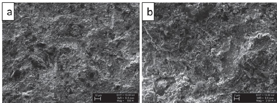
**Fig. 6:** Abrasive erosive wear of Z5 at 90° at magnification **(a)** 500X **(b)** 2000X
