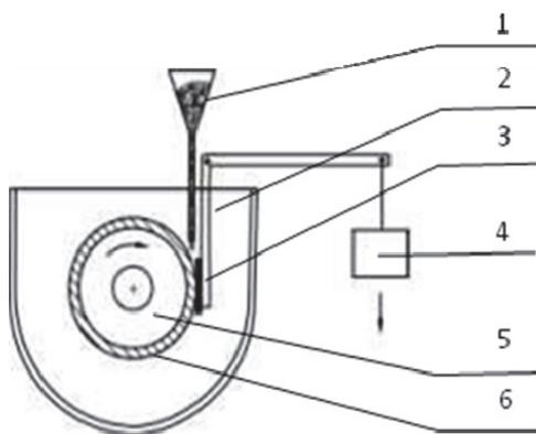
**Fig. 2.** Principal scheme of block-on-ring wear tester: 1 – abrasive particle vessel; 2 – specimen holder; 3 – specimen; 4 – weights; 5 – steel wheel; 6 – rubber wheel
