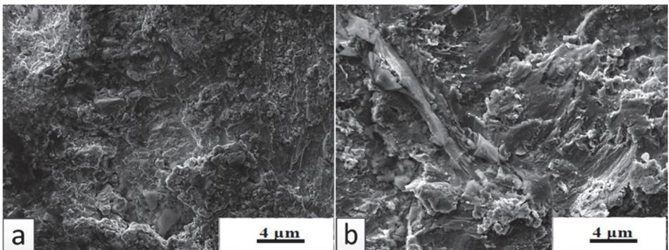
Figure 3.7 Topography of worn surfaces at A AEW  $\alpha=90^\circ$ ) of sprayed coatings from MATS hardmetal/cermet powders: a – WC-Co; b – Cr<sub>3</sub>C<sub>2</sub>-Ni
