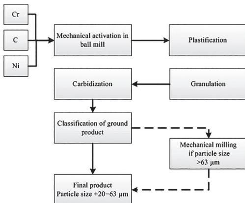
Fig. 1. Powder production via mechanically activated thermal synthesis.
