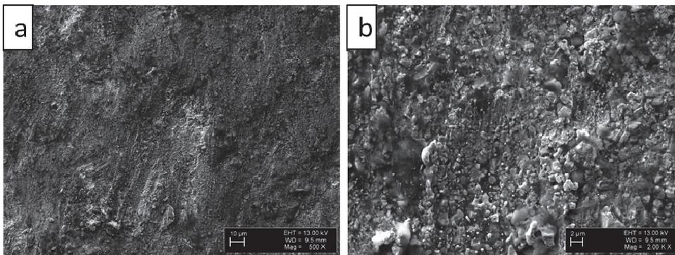
**Fig. 5:** Abrasive erosive wear of Z5 at 30° at magnification (a) 500X (b) 2000X
