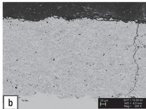
**Fig. 4.** Coating structures: (a) Cr<sub>3</sub>C<sub>2</sub>–Ni; (b) Amperit 588.074.
