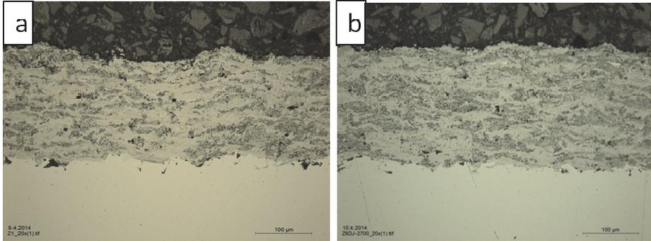
**Fig. 3:** Coating's structure (a) Experimental powder Z5 (b) Experimental powder Z6
