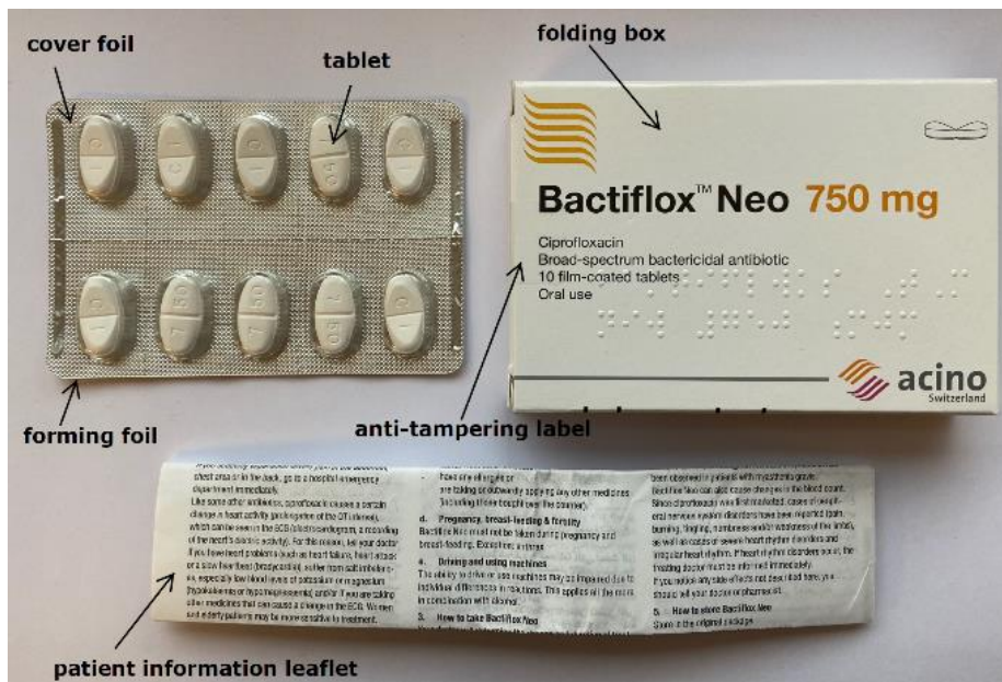
Figure 1.4 Blister packaging components
