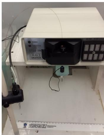
**Figure 9. CE-LED-induced fluorescence detector (TUT and LDI AS, Estonia)**
