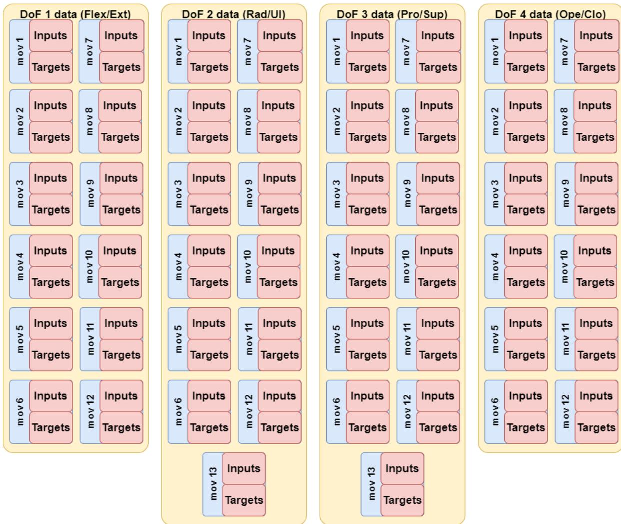
Figure 3.8 Movement-wise divided data sets. For every DoF, each motion data were segmented. The data consists of input and target sub-sets. Input data is compiled of extracted sEMG features. Target data consists of robot DoFs kinematics. Notations in parentheses represent user control motions responsible for corresponding DoF-s control: Flex – flexion, Ext – extension; Rad – radial deviation, UI – ulnar deviation; Pro – pronation, Sup – supination; Clo – fist closing, Ope - fist opening
