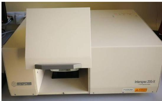
FTIR spectrometer, INTERSPEC 200-X
