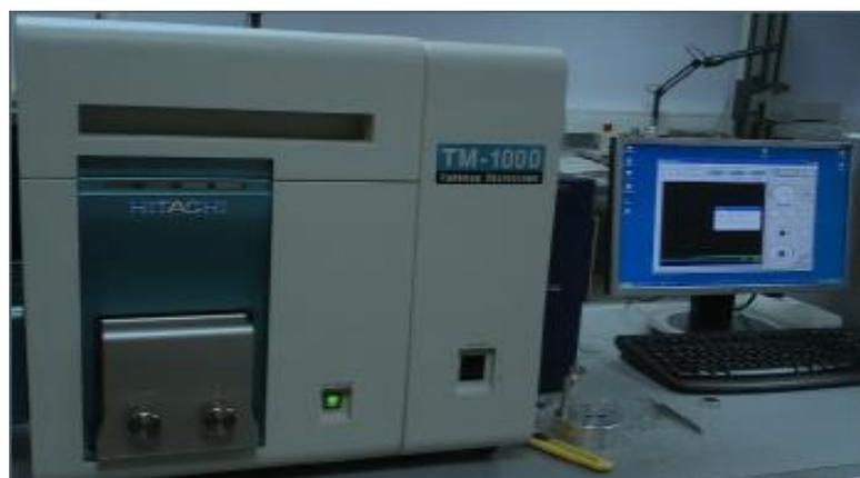
SEM microscope, TM1000, HITACHI
