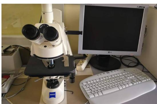
Optical microscope, Zeiss
