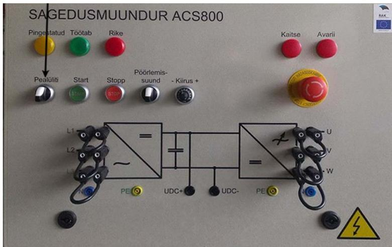
Figure 4.5 Control panel of ACS 800. An arrow shows the main switch
