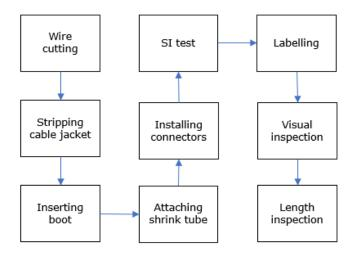
Figure 2.1 (Sample) production and testing process (Jem Electronics, 2018)
