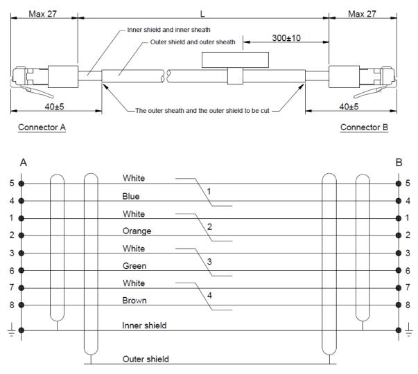
Figure 2.2 Drawing of RJ45-RJ45 signal cable with colour requirements and connection positions of the wires
