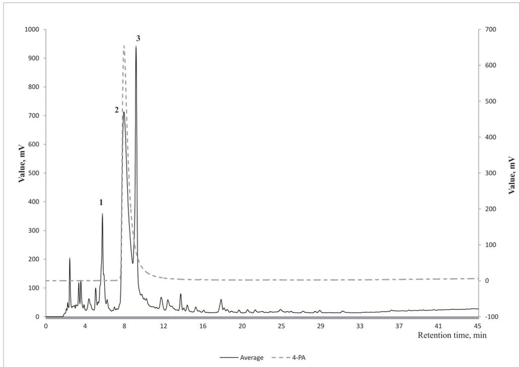
**Fig 2. Example of an averaged Ex320/Em430 nm chromatogram of the spent dialysate (N = 10).** Samples were collected 7–10 min after the start of the dialysis. Compound 2 was identified as 4-pyridoxic acid. Raised chromatogram is of a reference 4-pyridoxic acid solution (1  $\mu$ M).
