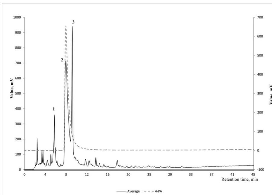
**Figure 4.** An example of an averaged EX320/EM430 nm chromatogram of the spent dialysate ( $N = 10$ ). Samples were collected 7–10 min after the start of the dialysis. Compound 2 was identified as 4-pyridoxic acid. Raised chromatogram is of a reference 4-pyridoxic acid solution.
