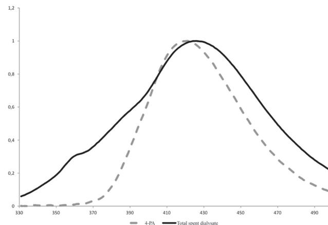
**Fig 1. Normalized emission spectra of spent dialysate (solid line) and 4-pyridoxic acid (dotted line) in  $\text{NaHCO}_3$ /acetate buffer pH 7.6. Excitation at 320 nm.**
