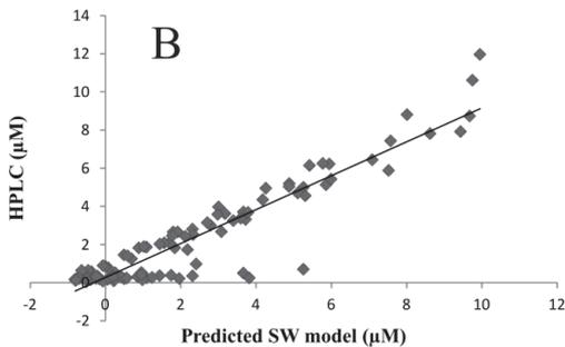
Fig. 2. 4-pyridoxic acid concentration determined by HPLC measurement and by the Ex/Em 310/460 nm model for the calibration (A) and validation (B) set, respectively.
