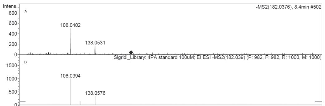
**Fig 3. Comparison of mass spectra (negative ionization) of A) biggest fluorescent peak (no 2, Fig 2) and B) 4-pyridoxic acid reference.**
