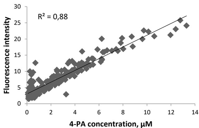
**Figure 5.** An example of correlation between the fluorescence intensity of the spent dialysate and the concentration of 4PA in the spent dialysate at EX310/EM460 nm ( $P < 0.0001$ ,  $N = 195$ ).
