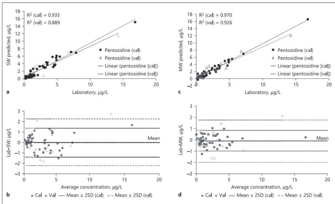
**Fig. 4.** Free pentosidine concentration determined at the laboratory and predicted by the SW (a) and MW (c) model, and Bland-Altman plot of the differences between Lab and SW (b), Lab and MW (d) concentrations. SW, single-wavelength; MW, multi-wavelength.
