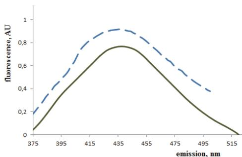
Fig. 3 Sediment's fluorescence spectrum (dashed line) compared with the spectrum of amyloid B2M (solid line) [8]
