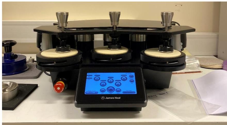
Figure 7.2.4 Martindale testing machine used for pilling and abrasion resistance tests.
