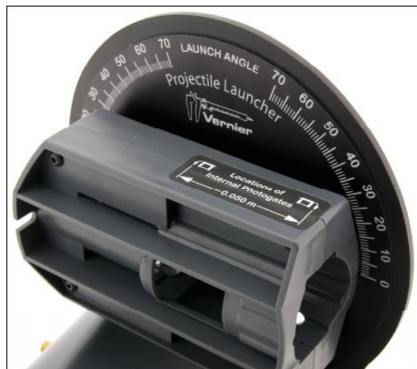
Figure 4.3 Locations of internal photogates [4]
