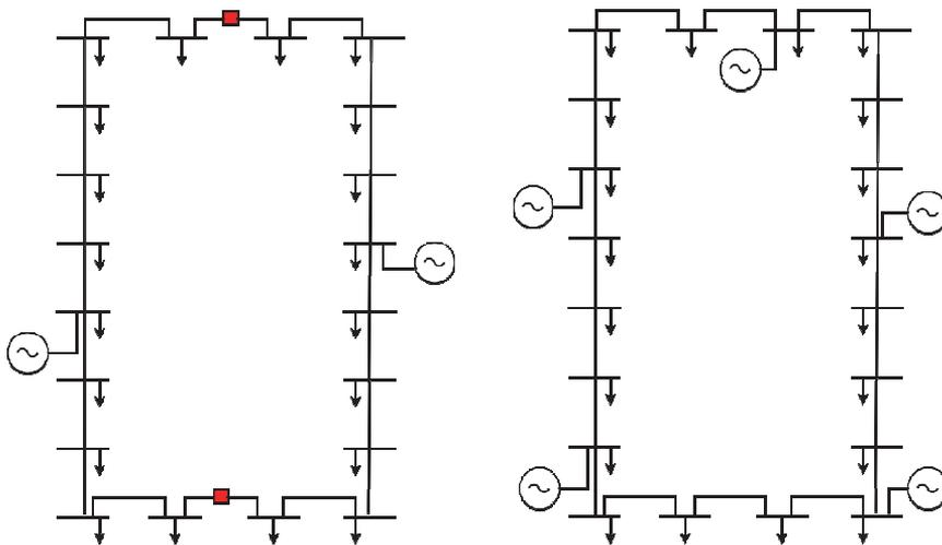
Figure 3.8. Models with 2x200 MW and 5x50 MW generators
