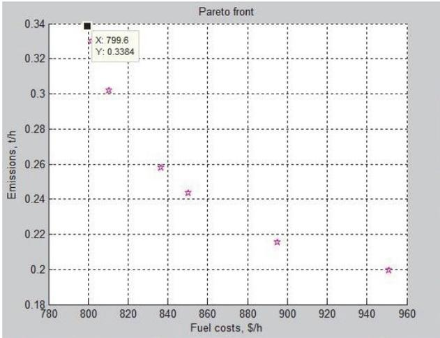
Figure 3.9. Results of multi-criteria optimization for model I
