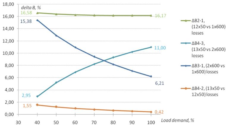
Figure 3.6. Difference in fuel consumption considering power losses. Model II. Fuel: coal
