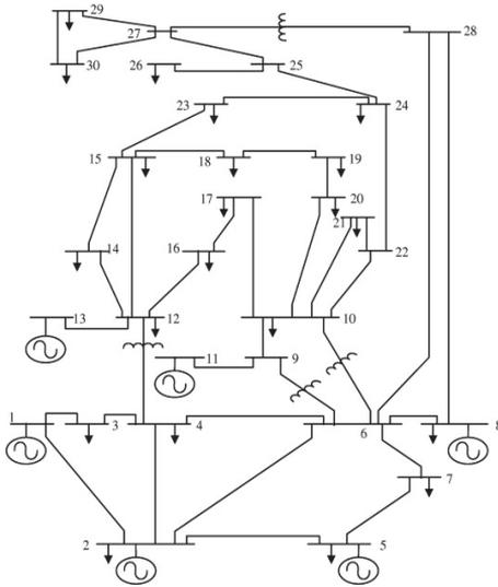
Figure 3.7. IEEE 30-bus test system[69]
