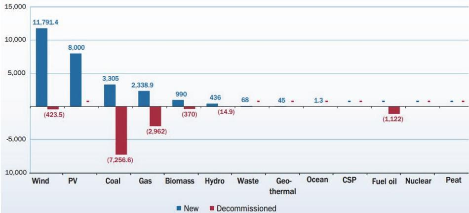
Figure 1.2. New installed and old deinstalled capacities in MW[2]
