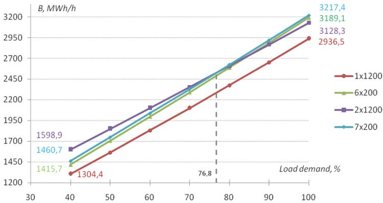
Figure 3.3. Fuel consumption without calculations of power losses. Model I. Fuel: coal.
