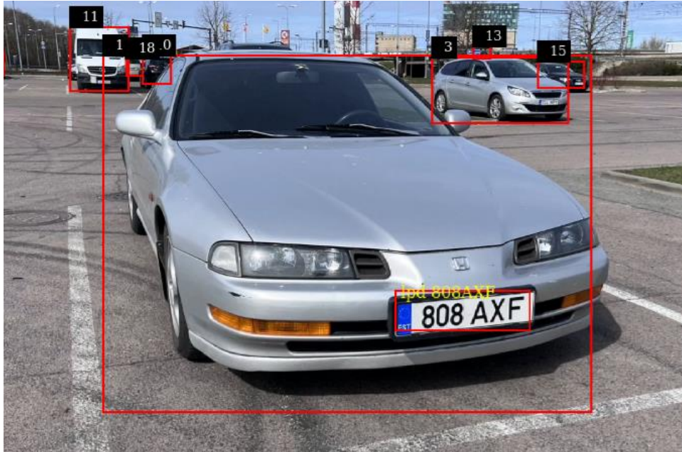
Figure 5 Multiple vehicles and license plate detected by NVIDIA LPR sample application
