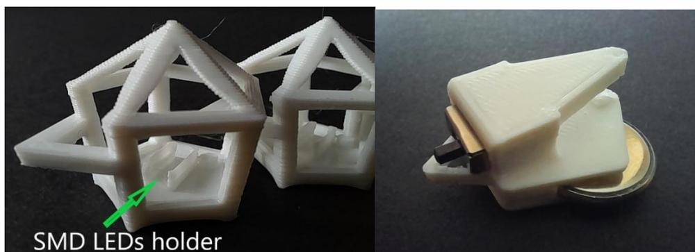
Figure 8. 2 Pentagonal box with LED holder (left); a battery and switch holder (right)
