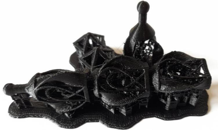
Figure 4. 19 The printing orientation of pentagon box design and lantern design using MakerBot printer.
