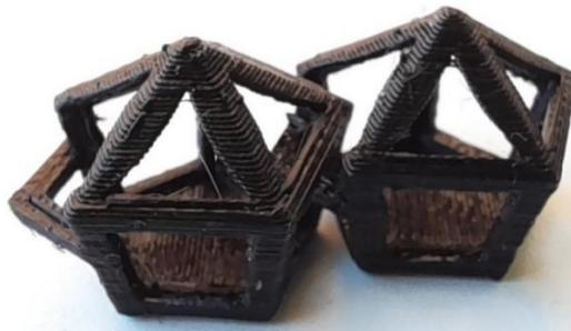
Figure 4. 20 The printing outcome of 12 mm pentagon box design after removing supports using MakerBot printer.
