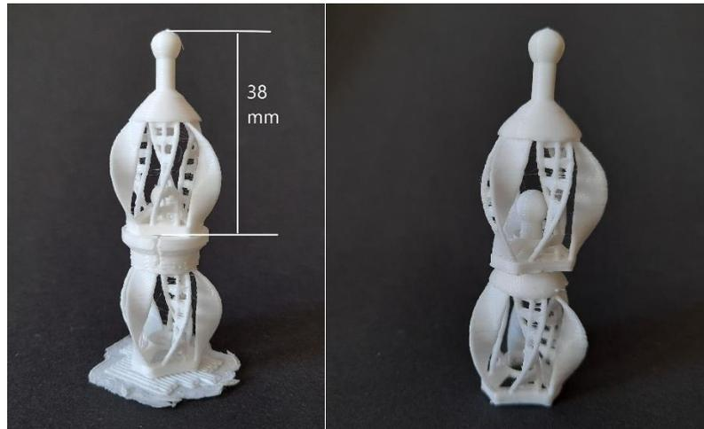
Figure 4. 23 The printing outcome of the lantern with designed manual supports (left) and after removing supports (right) using the Ender-3 FDM printer.
