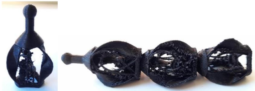
Figure 4. 21 The printing outcome of 38 mm lantern design in Z-direction (left) and XY-direction (right) after removing supports in the MakerBot printer.
