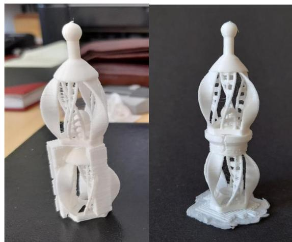
Figure 4. 24 The comparison between the auto-generated printing supports (left) and manual-designed printing supports (right).
