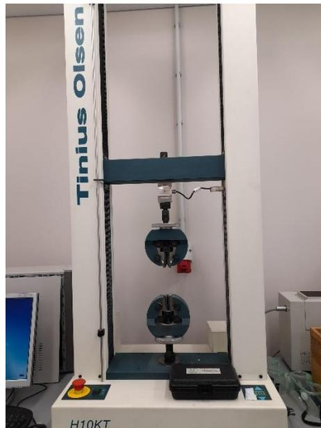
Figure 7. 1 Tinius Olsen tensile testing machine.
