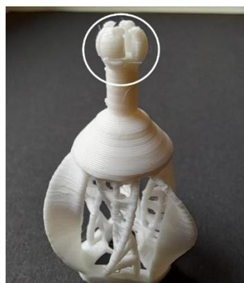
Figure 4. 26 The printing outcome of the lantern with snap-fits design with the cutting of sphere head using Ender-3 FDM printer.
