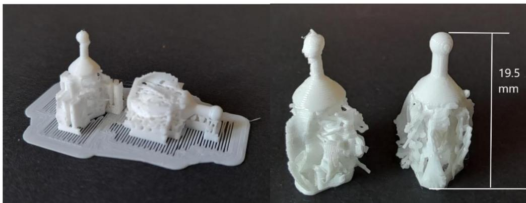
Figure 4. 17 The printing outcome of lantern design with supports (left) and after removing supports (right) using Ender-3 FDM printer.
