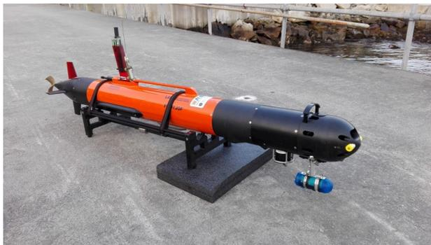
Figure 15 – LAUV Fridtjof with attached DPSSv2 [publication V]. The AUV used DVL, GPS and INS for navigation and the DPSSv2 was sampling independently.
