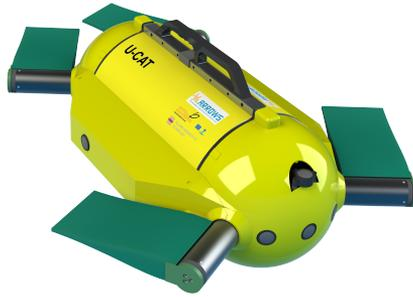
Figure 23 – **Rendering of bio-inspired AUV U-CAT with 4-fin propulsion.** The vehicle is shown in FAST mode configuration where all flippers point towards the back of the robot when not actuated. This is the configuration that will be used throughout the subsequent controller development.
